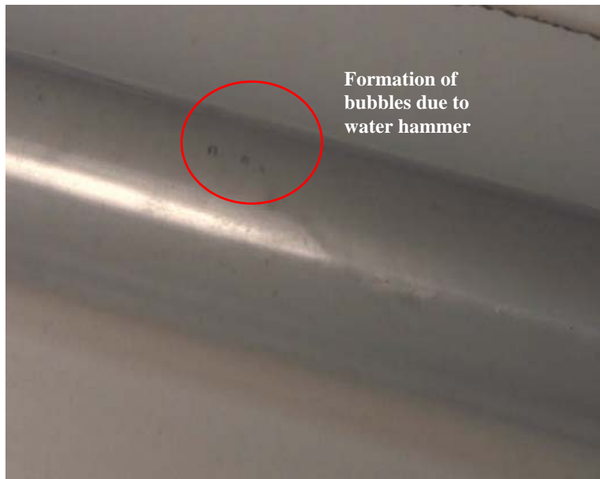
Figure 4. Water hammer induced homogenous gaseous cavitation.
