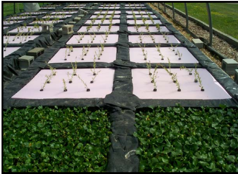
Figure 1. The modified hydroponic system used to evaluate woody shrub accumulation of N and P. (In the foreground are the water hyacinths used to develop the protocol.)
