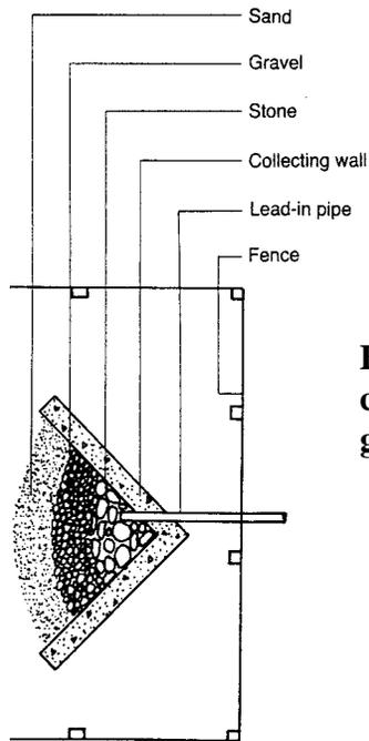
**Backfill the area from the channel to the cut-off wall with graded sand, gravel, and stone.**
