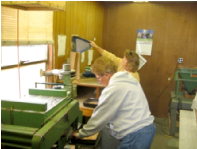
Figure 2. Shelling and grading to determine market grade and value according to the loan rate.
