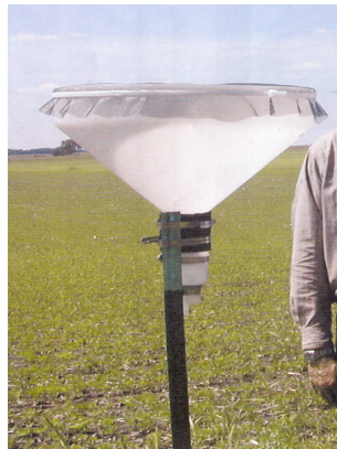
Fig. 4. Wet deposition trap.
