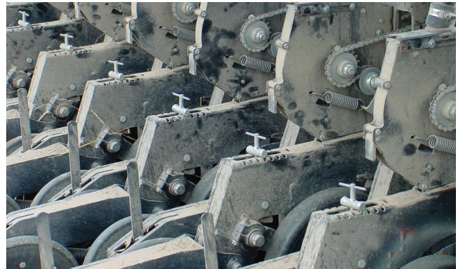
Figure 5. Seed metering for seed singulation on a grain drill. Meter device is shown with gear and chain drive (see fig. 6 for location).
