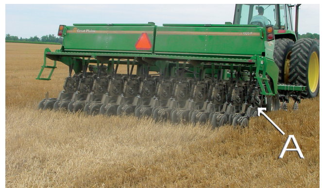
Figure 6. Precision seeding system with seed meters close to the ground ("A" marks the metering device).
