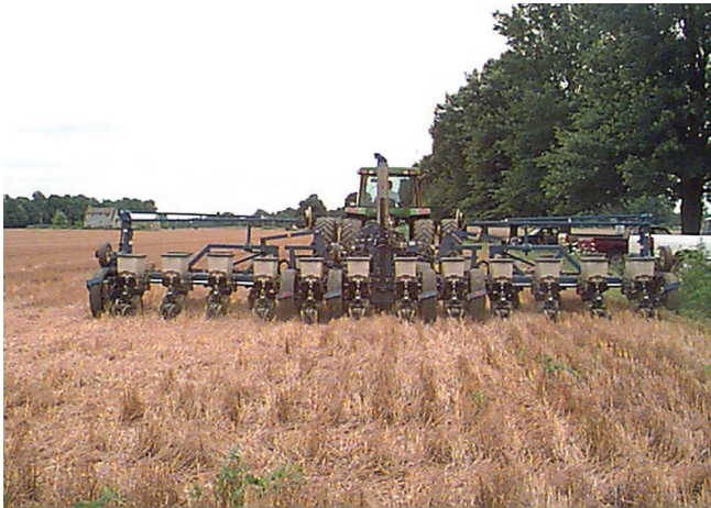
Figure 7. Planter equipped with extra planter boxes to plant 15-inch rows.
