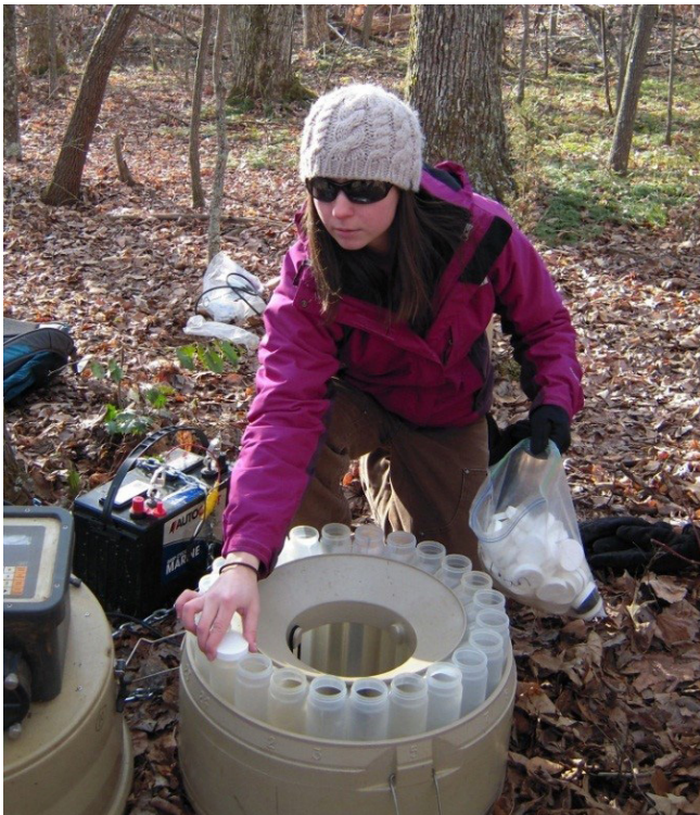
Figure 5. An automated water sampling device collected daily samples for one year.
