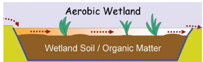
Figure 2. Simplified cross-sectional view of an aerobic wetland. These systems can treat mildly acidic, circumneutral, or alkaline waters that contain dissolved metals such as Fe (iron) which can be transformed to the solid phase via oxidation. Aquatic plants such as cattails translocate O_2 to the subsurface through their roots, which aids metal oxidation. The aquatic plants also help to prevent channelization of the waters flowing through the wetland, slowing water velocities and aiding solid-phase metal removal via sedimentation.
