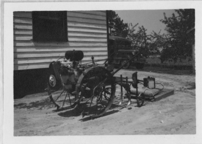
Fig. 8 - Equipment Set-up With Steel Wheels.
