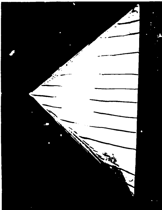
Fig. 7 Oil flow patterns, \alpha = 40^\circ , \beta = 0^\circ .
