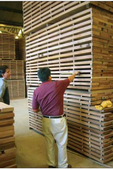
Omar Espinoza takes measurements during an evaluation of a Bolivian lumber drying operation, which will be used to identify opportunities for improvement.
