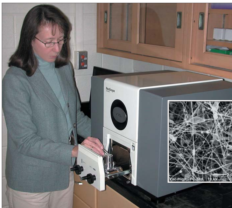
Audrey Zink-Sharp demonstrates the new scanning electron microscope, which produced this high-magnification image of cellulose filaments.
