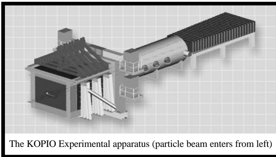
The KOPIO Experimental apparatus (particle beam enters from left)
