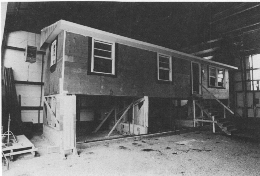
Fig. 11. MODULE ELEVATED FOR FLOOR LOAD-TESTING
