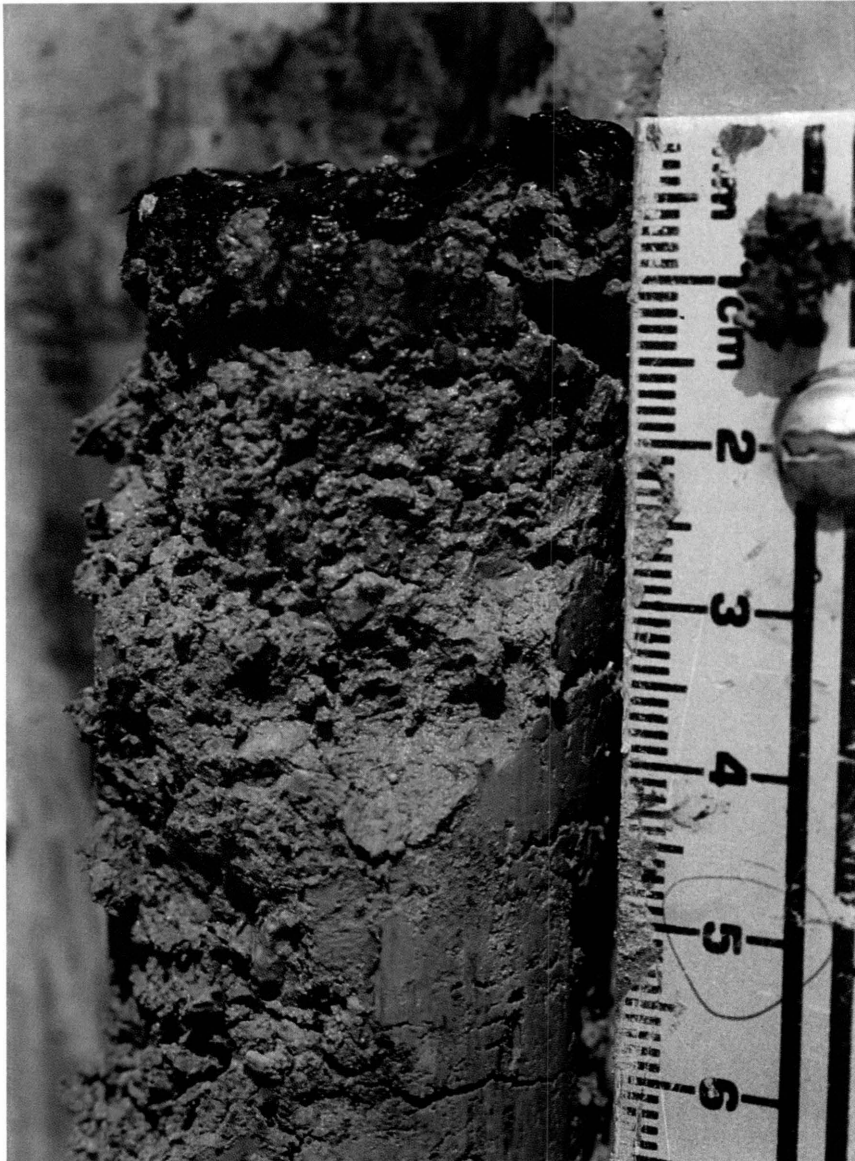
Plate 6. Top 10 cm of soil core sample below trench 6, Site 3. Note the mat of organic matter which has accumulated at the gravel-soil interface under ponded conditions.
