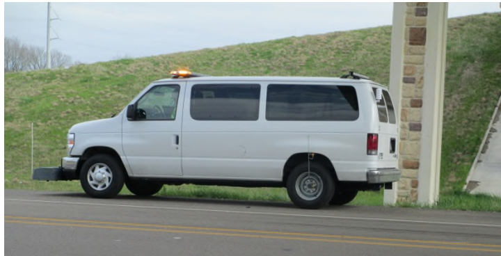
Figure 1. Inertial profiler equipped with a light bar and a directional warning light.
