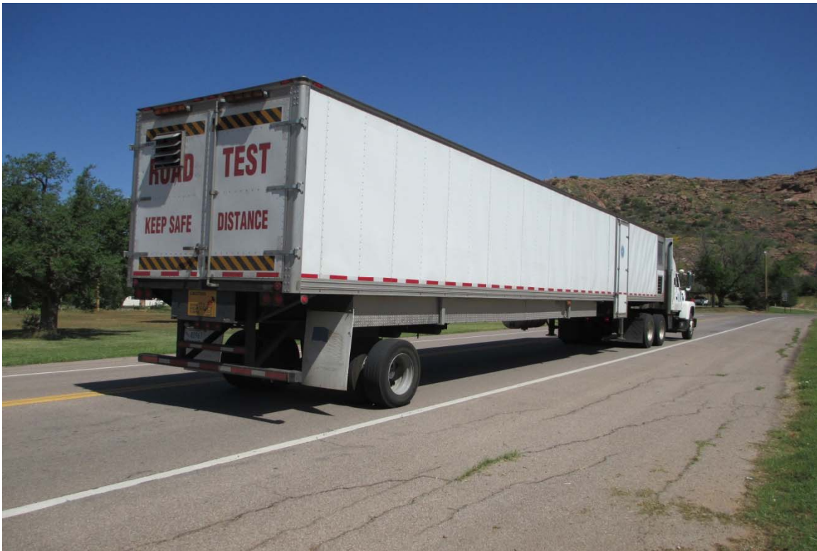
FIGURE 5. ARA Rolling Wheel Deflectometer (provided by Doug Steele of ARA)
