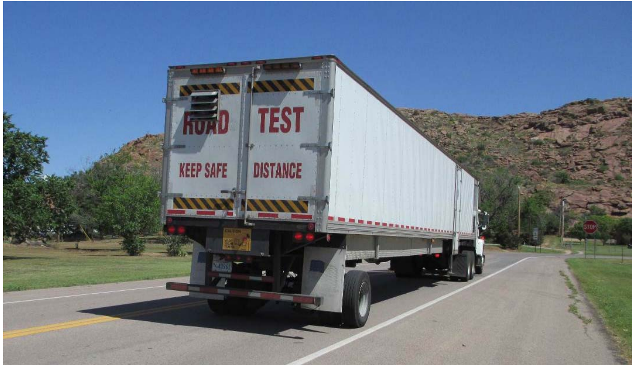
FIGURE 1 The RWD uses a series of lasers mounted in the passenger wheelpath to measure pavement structural response produced by its 18-kip trailer axle.
