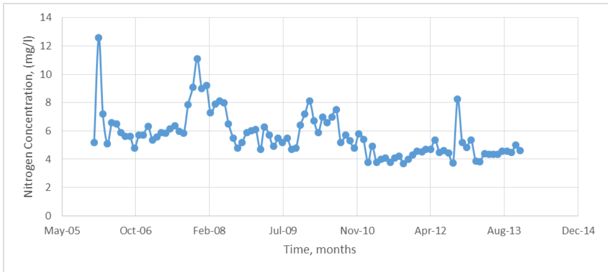
FIGURE 15. Leesburg WWTP Nitrogen Concentrations with BNR Technology, 2006-2013
