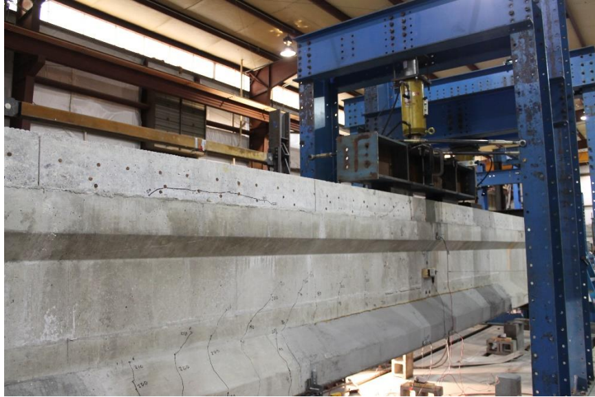
Figure 3.32: Cracking Patterns near Maximum Applied Load in Test 5
