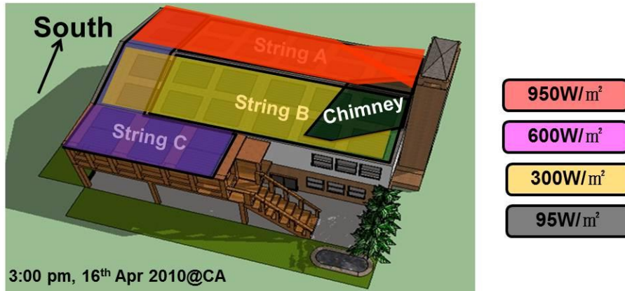
Figure 3.10 Case study of a severe mismatch for a residential PV system
