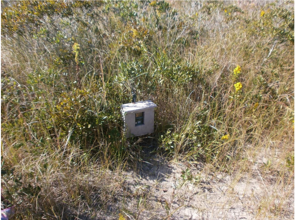
S5. Image showing Reconyx PC90 professional covert infrared cameras (Reconyx, Inc., Holmen, Wisconsin, USA) placed in a wooden box approximately 20 cm above the ground and attached to a metal pole sunk into the sand.
