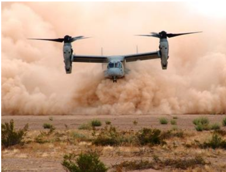
Figure 1. An example of V-22 Osprey operating at low altitude in particle-laden environment. [Dept. of Defense, Used under fair use, 2015]
