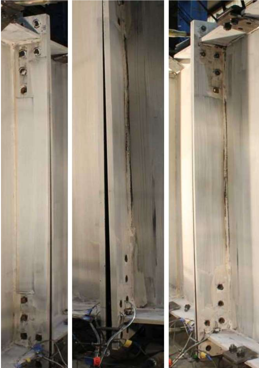
Figure 6-43 Three views of the specimen 12B-MRE 1/3-4W/2W-0.75-1.00-60 at the end of the test
