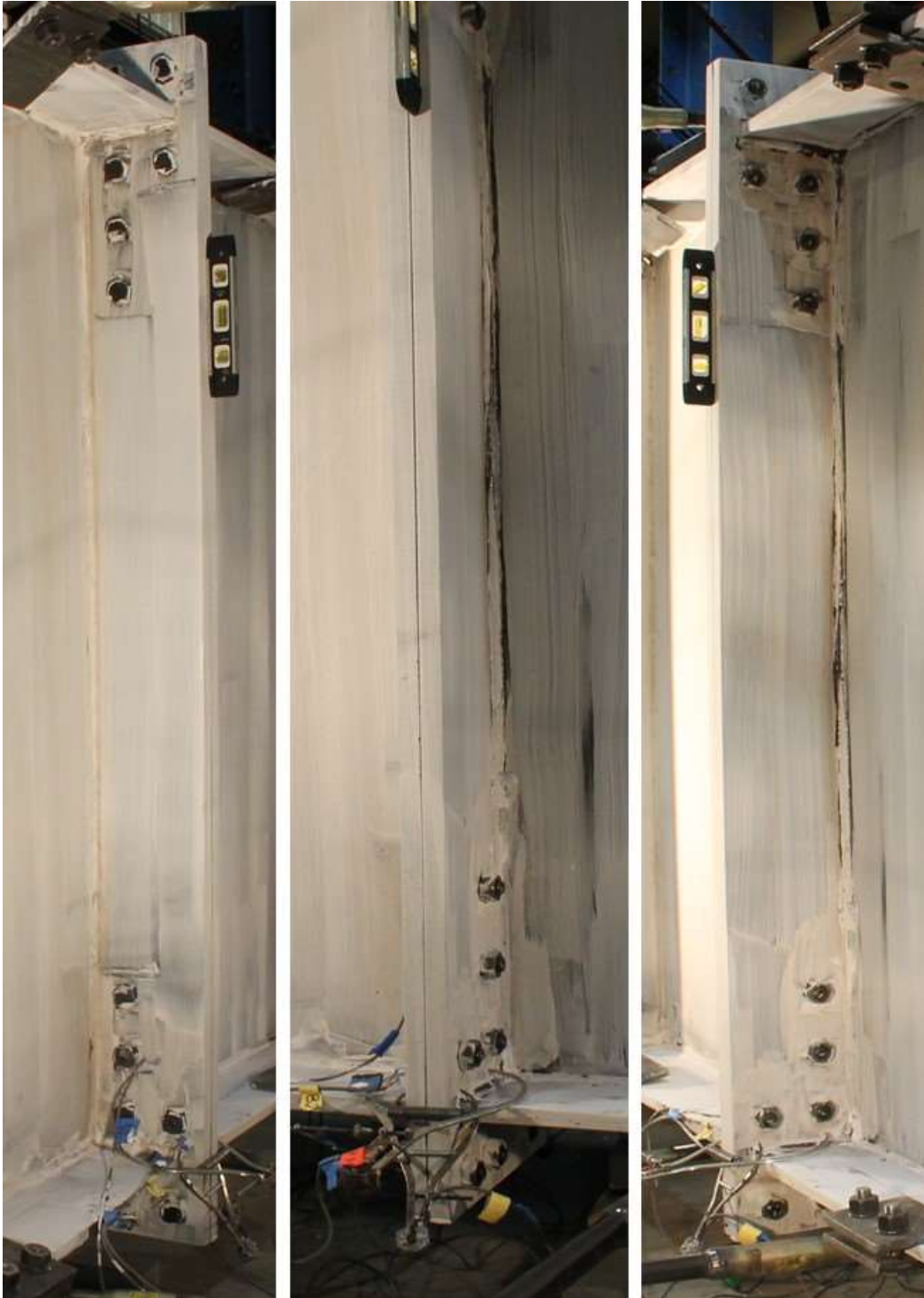
Figure 6-42 Three views of the Specimen 12B-MRE 1/3-4W/2W-0.75-1.00-60 at the start of the test
