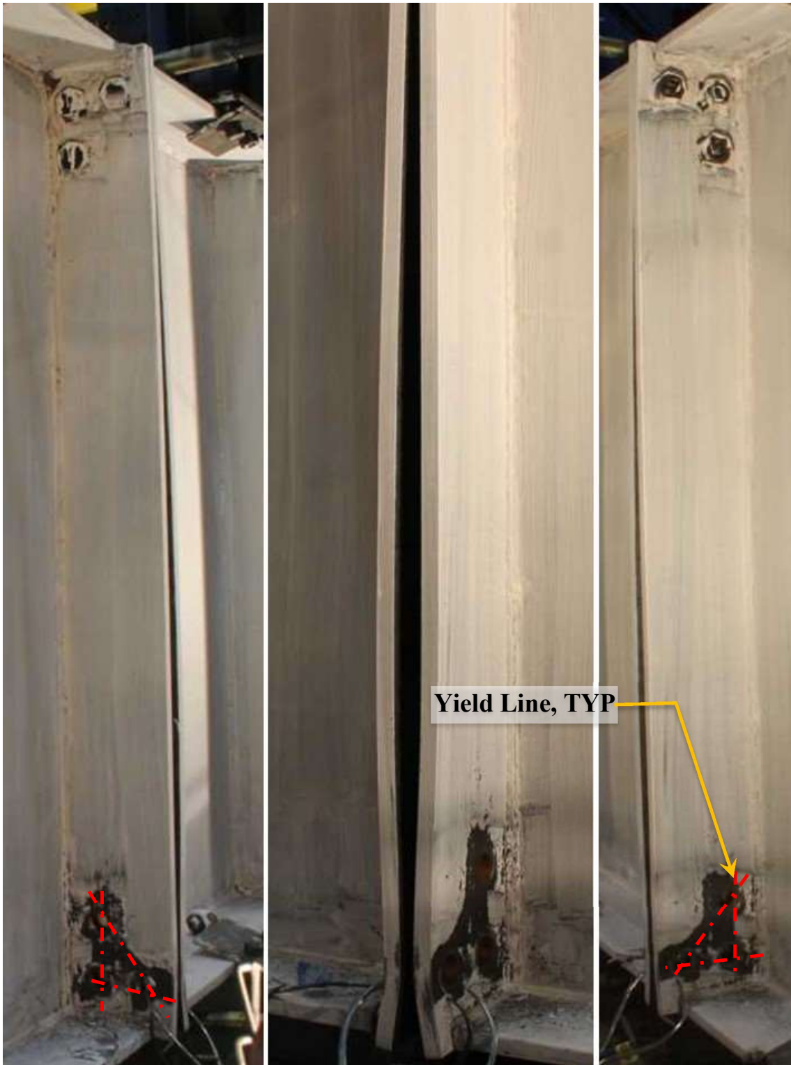
Figure 6-15 Three views of the specimen 6B-4W/2W-1.125-0.75-60 at the end of the test
