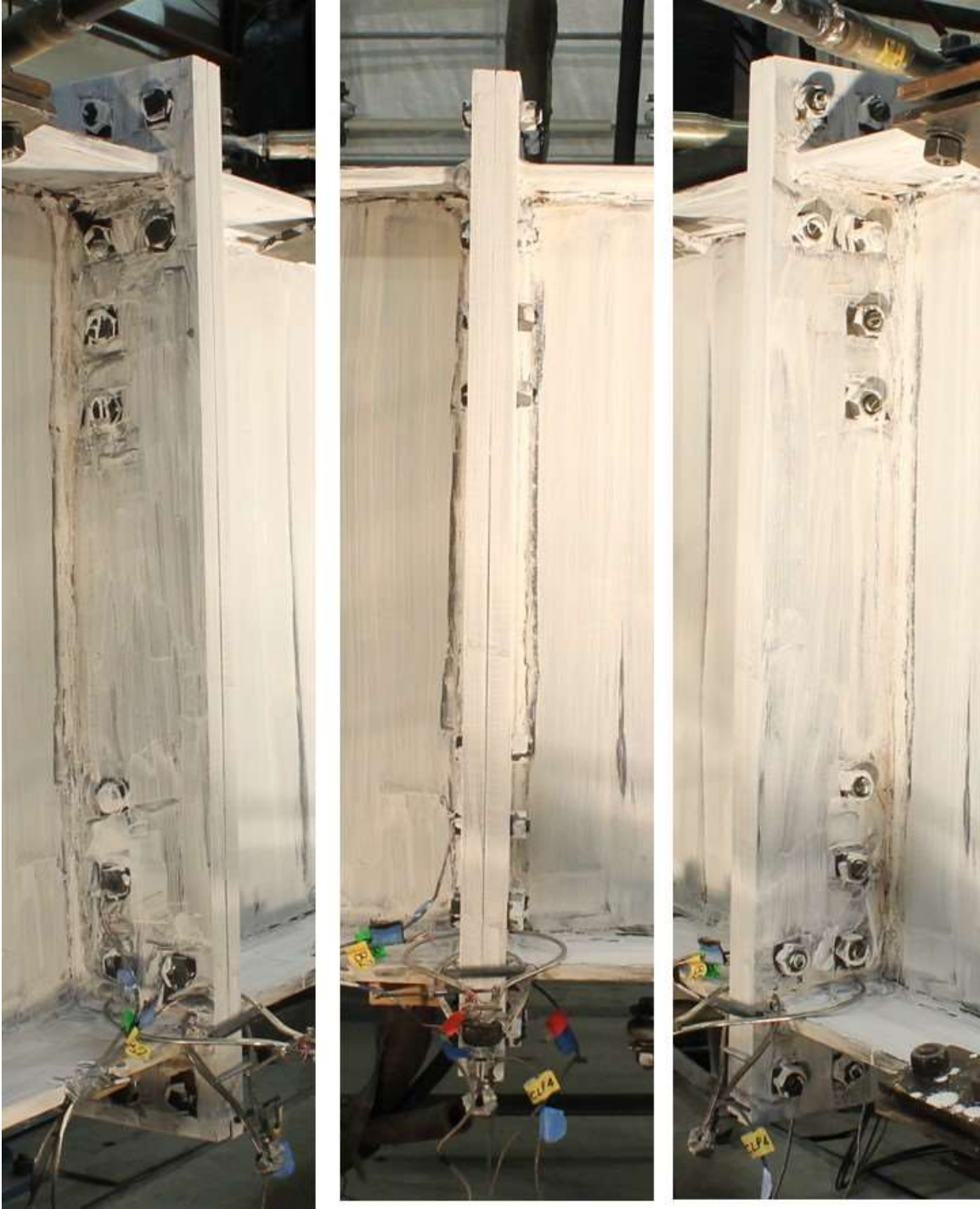
Figure 6-29 Three views of the Specimen 12B-MRE 1/3-4W/2W-0.75-1.00-36 at the start of the test
