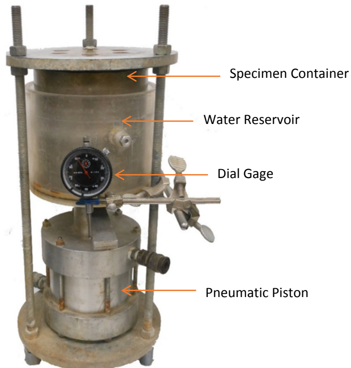
Figure 5.15 Batch consolidometer
