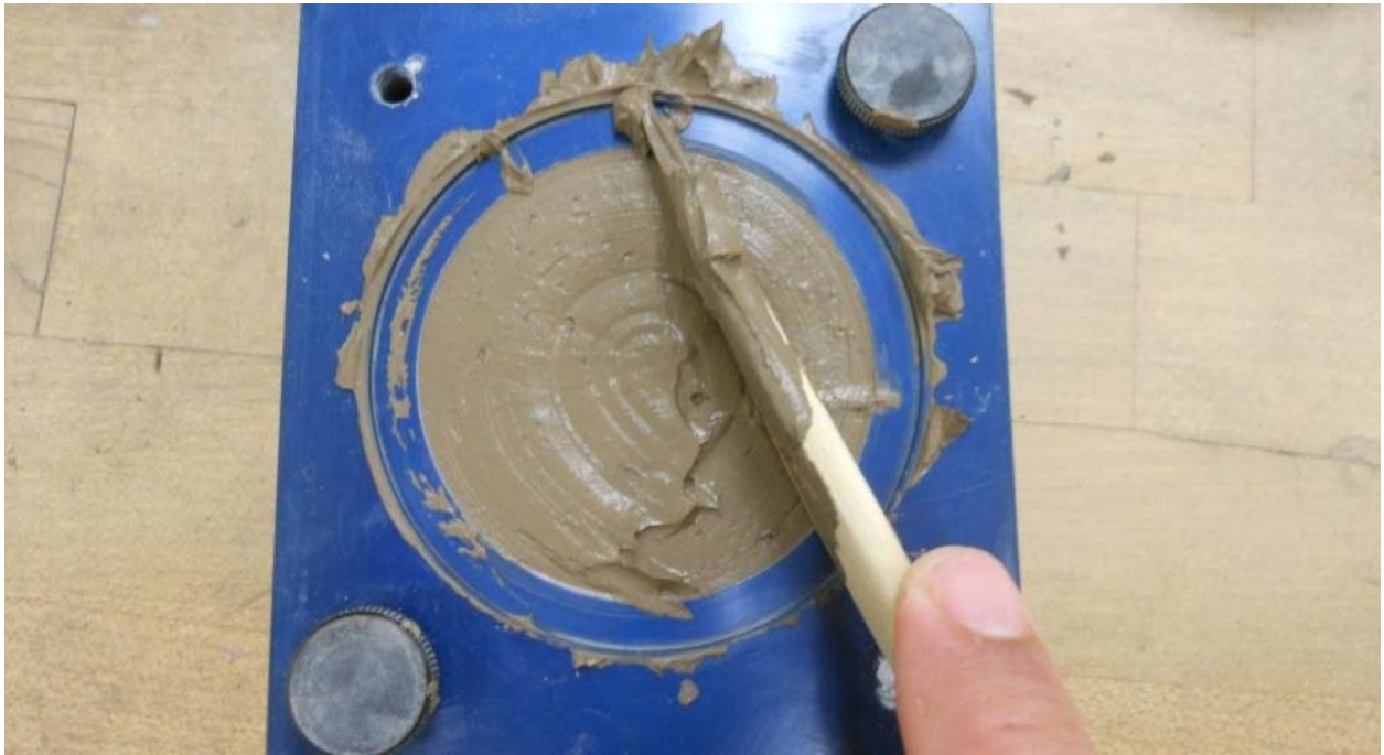
Figure 5.21 Test specimen being leveled with the top of the shear box.
