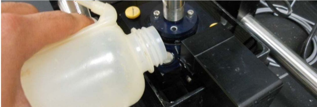
Figure 5.23 Distilled water being added to the water bath in the direct shear device.
