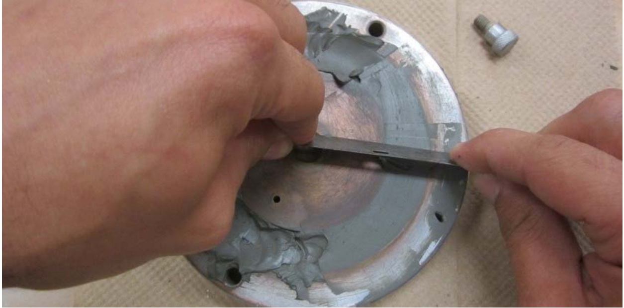
Figure 5.25 Ring shear test specimen being leveled with the top of the specimen container.
