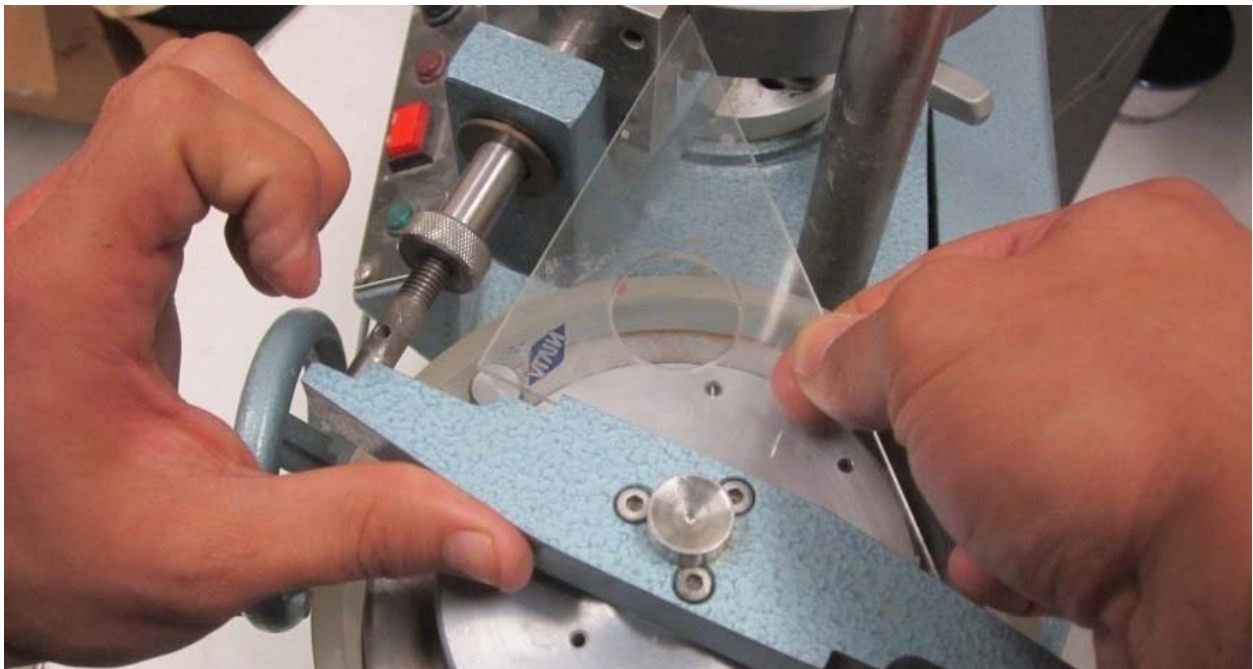
Figure 5.28 Verification of the orthogonality between the top platen and the proving rings.
