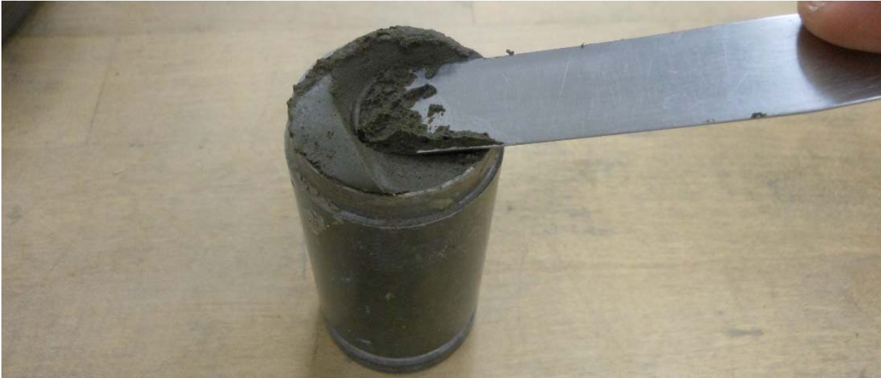
Figure 5.34 Packed specimen being formed.
