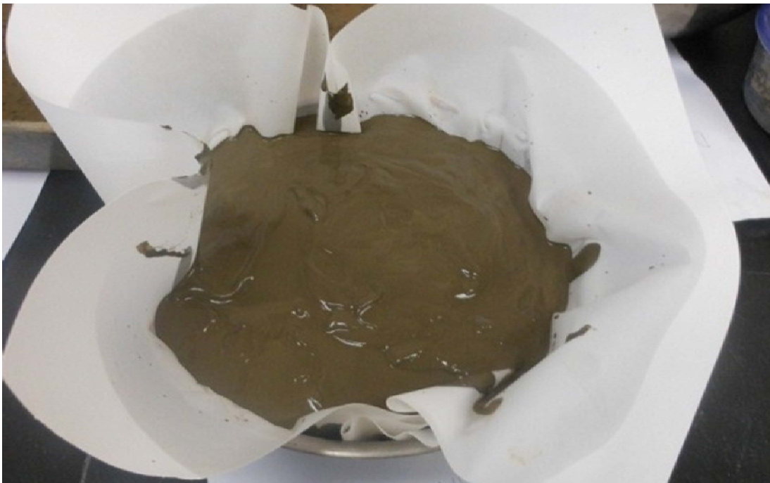
Figure 5.5 Soil sample being air-dried in a bowl with filter paper.
