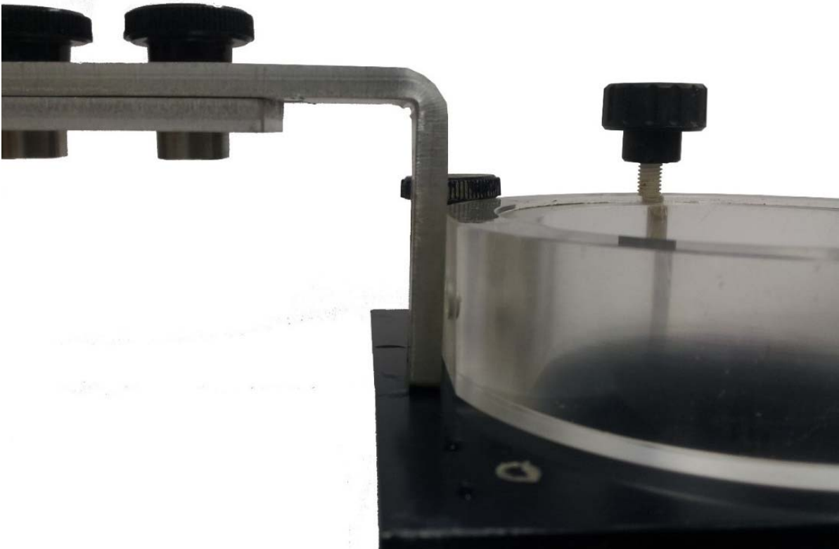
Figure 5.9 Connection between the yoke and the direct shear box.
