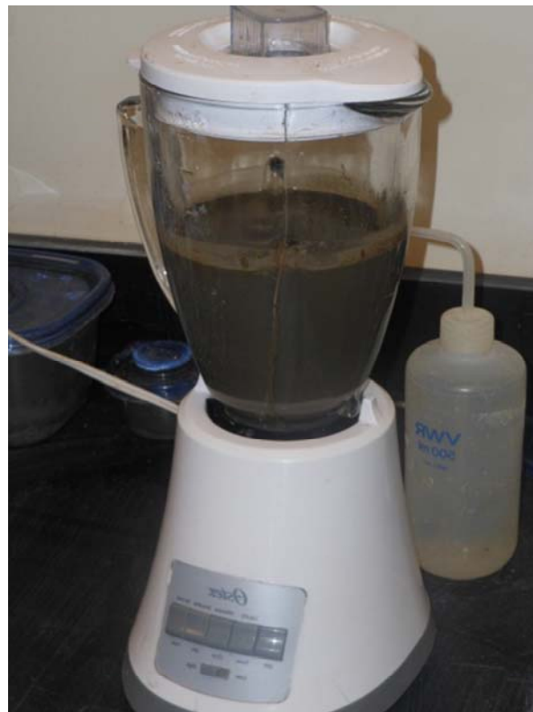
Figure 5.3 Soil sample ready to be blenderized.
