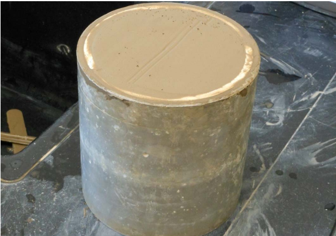
Figure 5.32 Batch consolidometer's specimen container full with soil.
