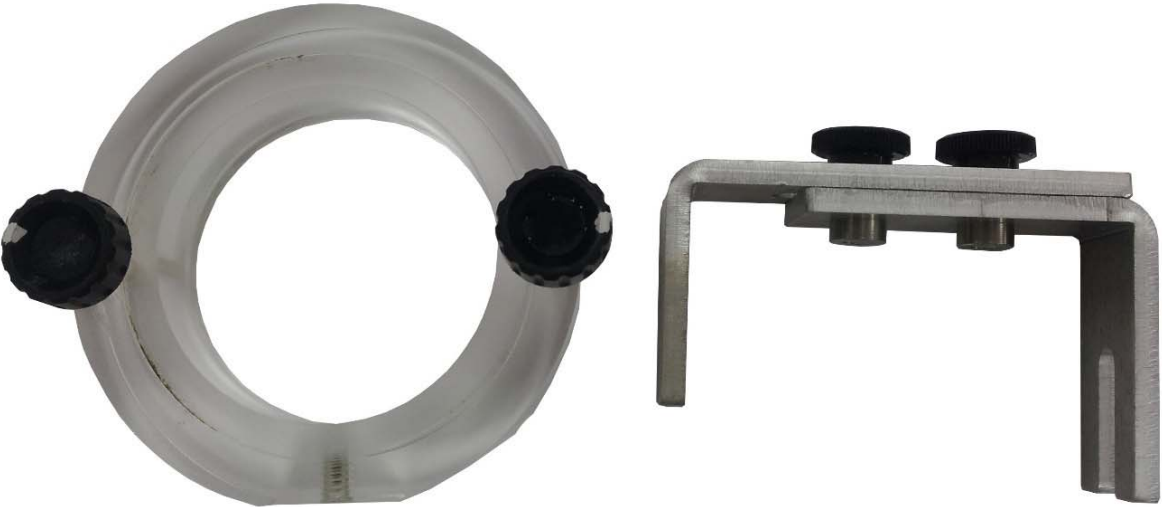
Figure 5.8 Modified direct shear box top half and yoke.
