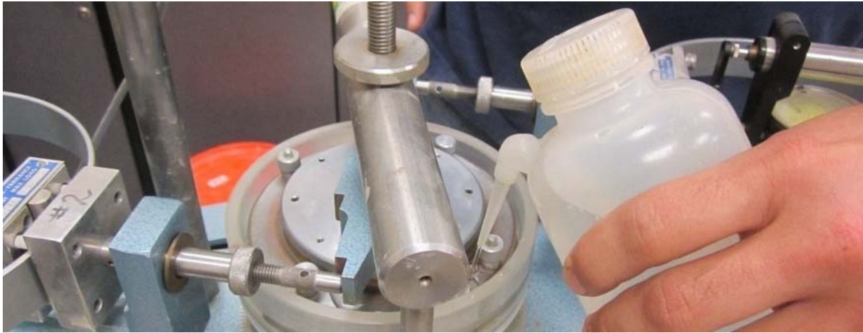
Figure 5.29 Distilled water being added to the water bath of the ring shear device.
