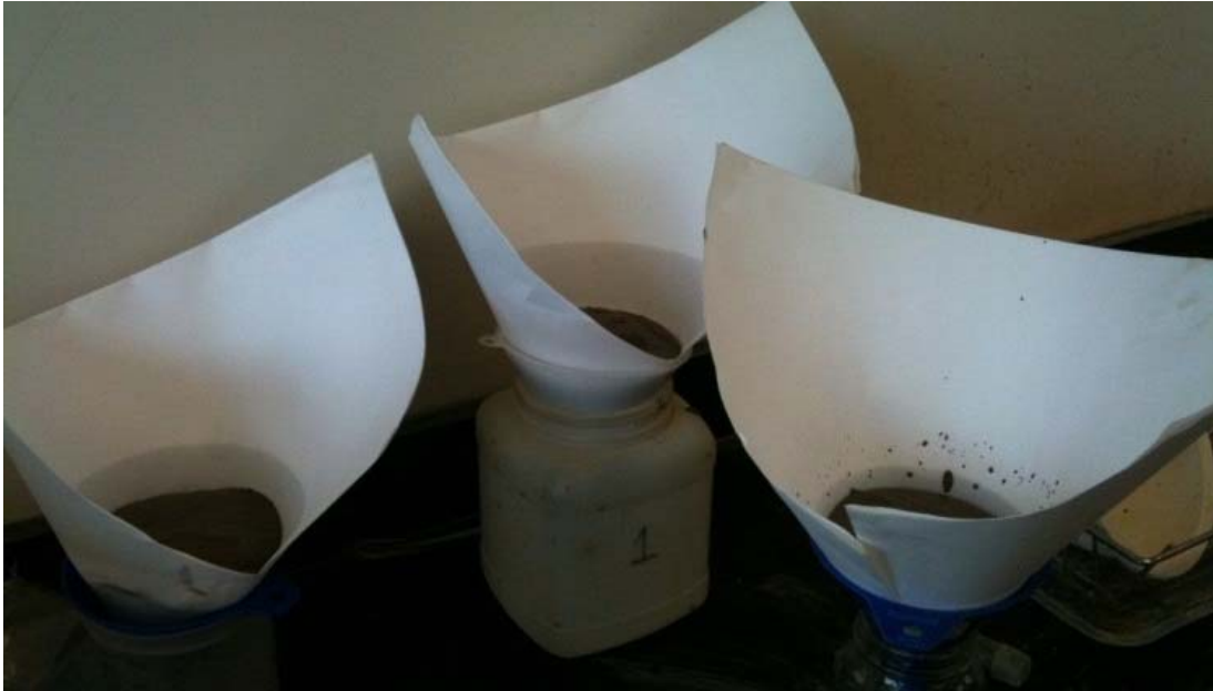
Figure 5.4 Soil sample being air-dried in funnels with filter paper.
