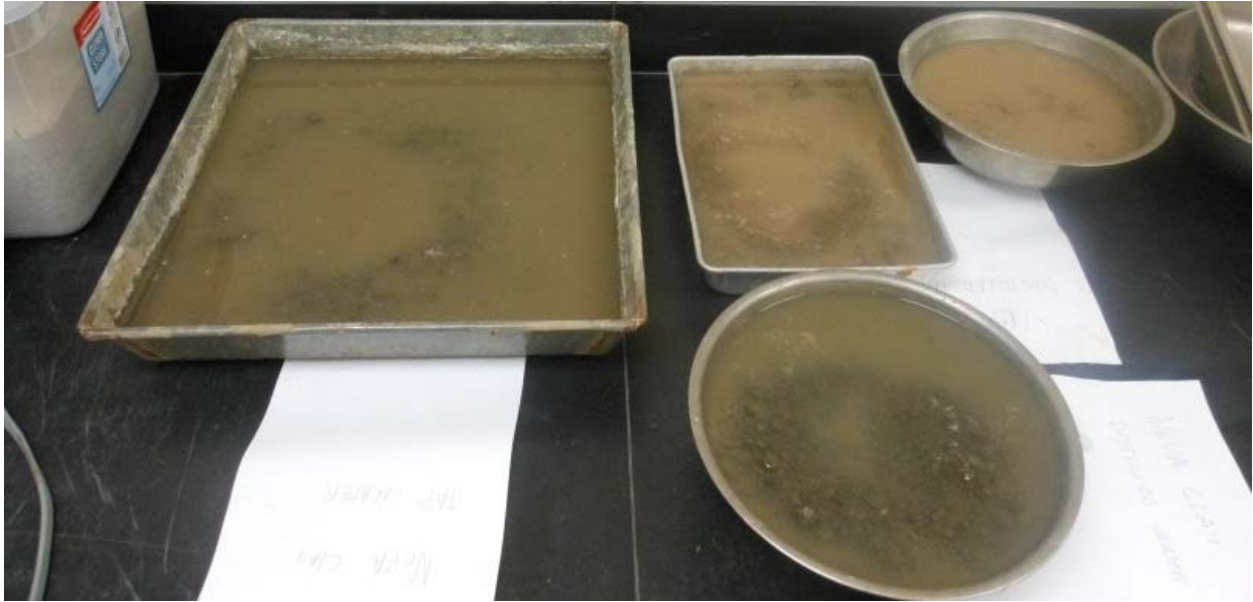
Figure 5.2 Soil samples allowed to soak in water.
