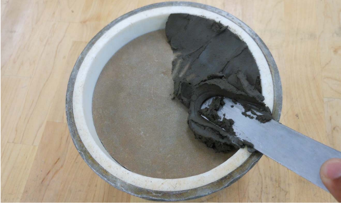
Figure 5.31 Batch consolidometer's sample container being filled.
