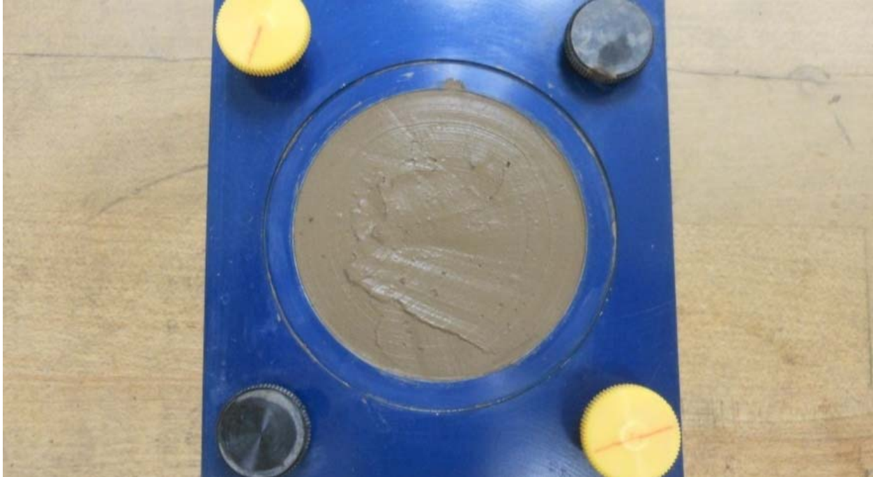
Figure 5.22 Specimen container ready to be weighed and placed in the direct shear device.
