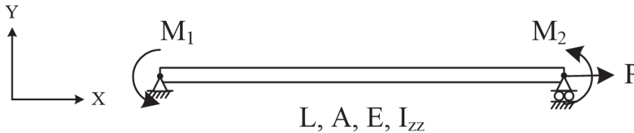
Figure 2-17: Simply Supported Beam-Column with Axial Load and End Moments
