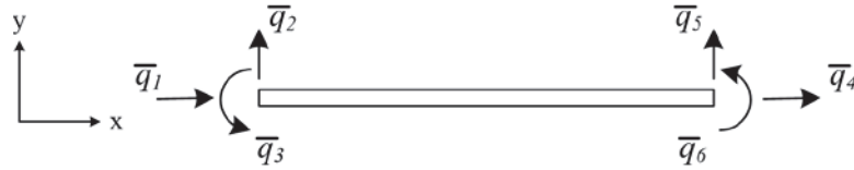
Figure 2-2: Planar Beam-Column Element
