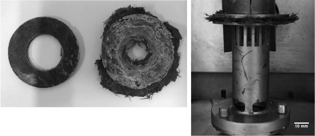
Figure 4.3: A 50 mm donut-shaped sample at 20 wt% carbon fiber – polypropylene prior to sample loading in a cone-and-plate rheometer (left), sample removed from rheometer at 60 strain units (middle) and the same sample shown in the rheometer prior to removal (right).
