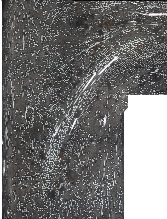
Figure 3-6: 50 wt % glass fiber high viscosity polypropylene at the gate-mold interface.
