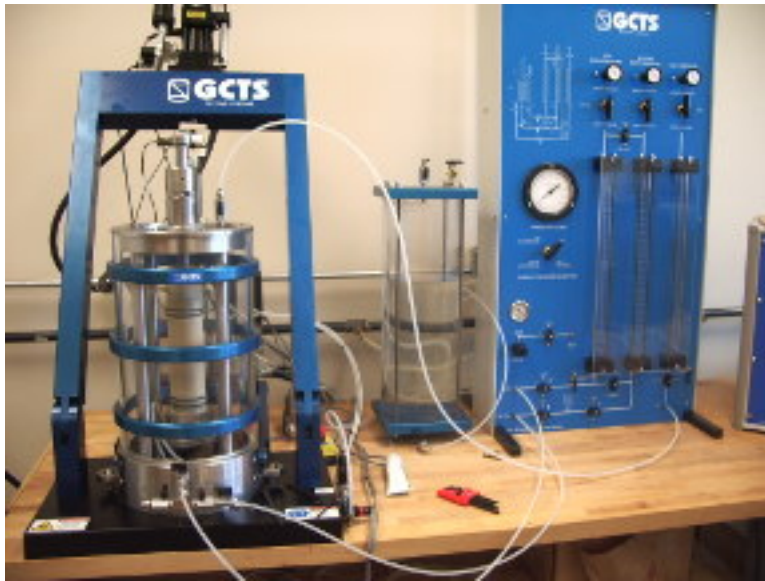
Figure 3.6: The GCTS testing apparatus used for this study with triaxial specimen. (Modifications not shown.)
