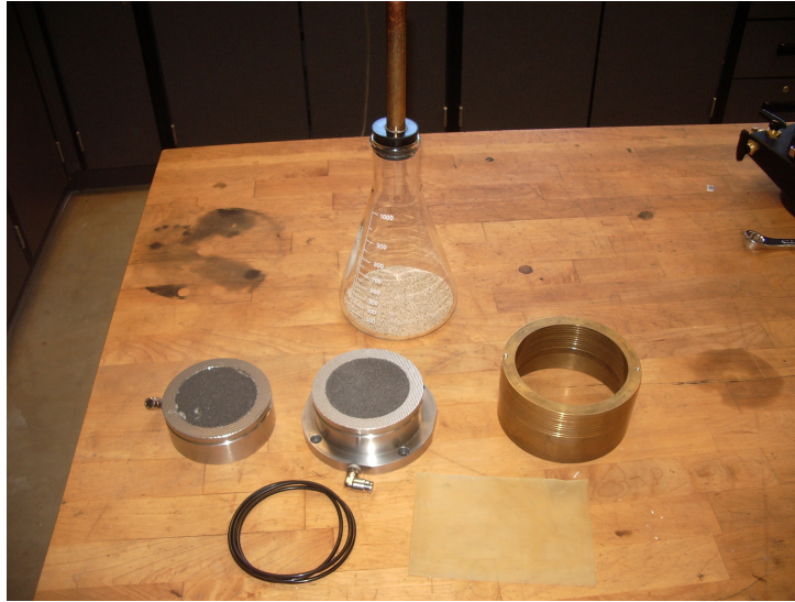
Figure G.5: Clockwise from left: top platen, flask with stopper and spout, brass confining rings, membrane, o-rings, and, at center, bottom platen.
