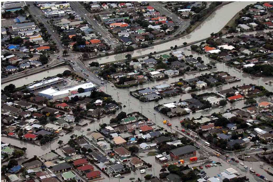
Figure 1.2: Liquefaction during the Christchurch earthquake sequence led to the condemnation of entire neighborhoods (NZDF 2011). [Fair Use]
