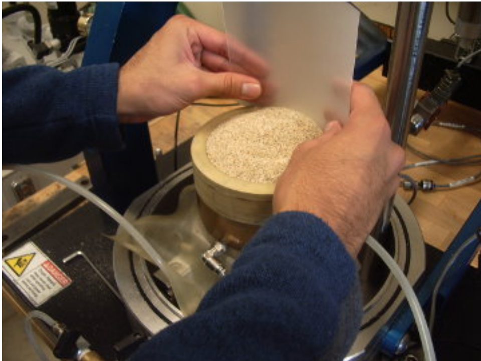
Figure D.4: Removing excess sand from a liquefaction-evaluation specimen.
