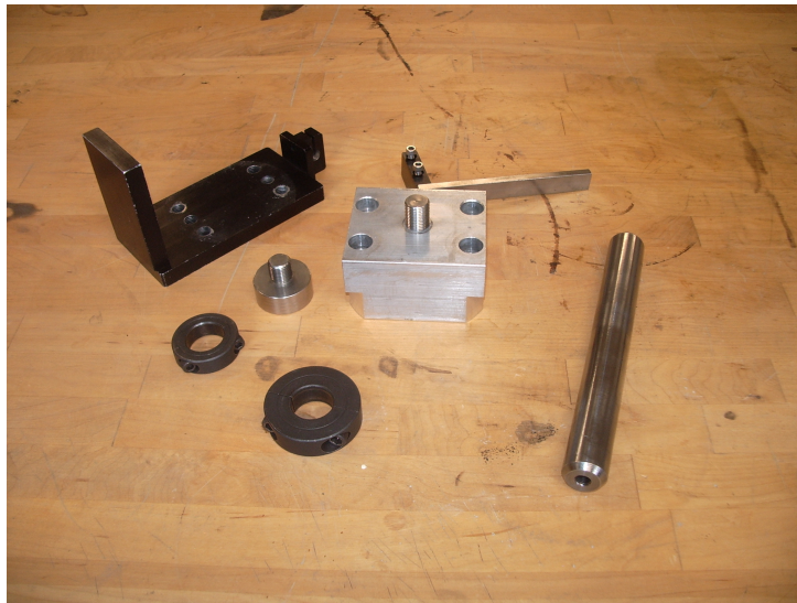
Figure G.6: Clockwise from the top left: the internal LVDT assembly, the internal shear LVDT reaction plate and bracket, the normal piston, large and small shaft-locking collars, and the normal actuator contact plate. In the center is the top-platen-to-normal-piston block.
