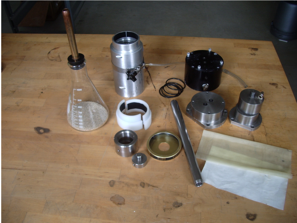
Figure H.5: Assorted other parts used in a triaxial test. Clockwise from the left: sand-filled flask with spout, 2.8-inch triaxial mold, o-rings, black triaxial pedestal, additional pedestal for 2.8-inch specimens, the top and bottom platens, a latex membrane, a piece of filter paper, the normal piston, a pi tape, the normal actuator contact plate and mating collar, and a mold extender.
