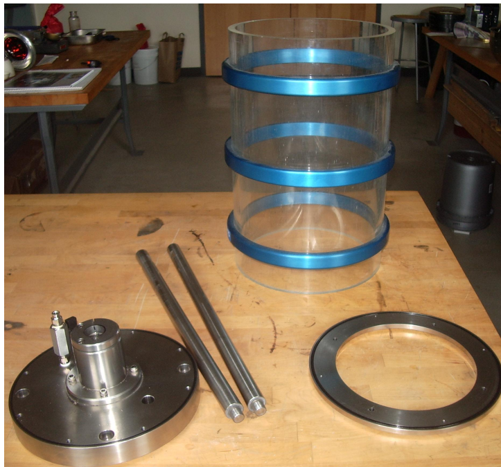
Figure H.3: Other parts of the cell. Clockwise from bottom left: the top cap, two of the four columns, the cell wall, and the top ring.
