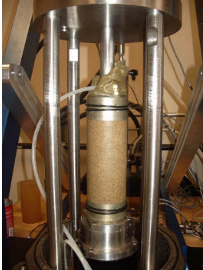
Figure 2.1: Triaxial specimen of Monterey 0/30 sand with vacuum applied.
