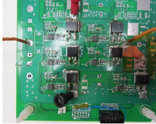
Figure 2.29 250W micro-inverter hardware prototype
