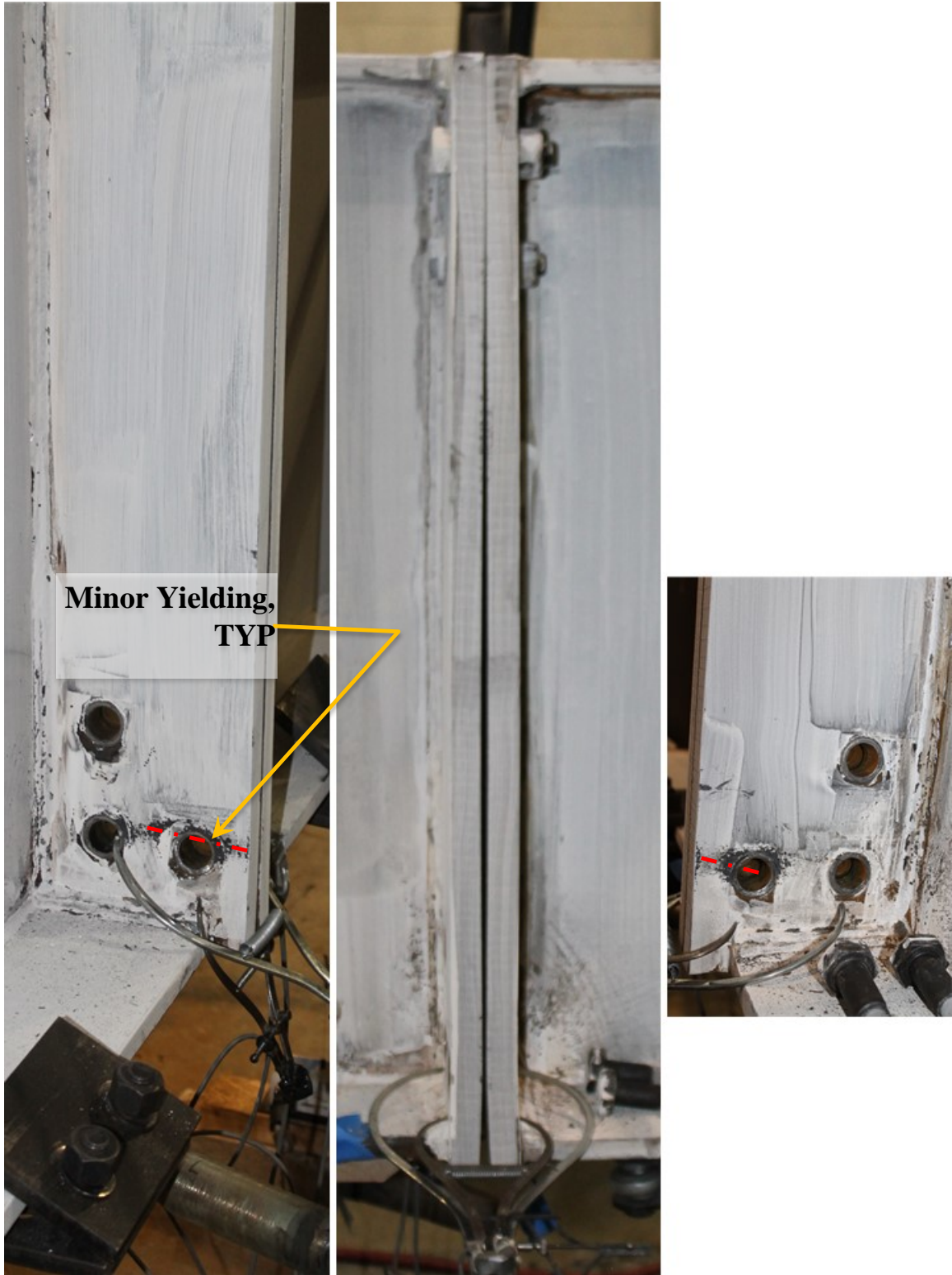
Figure 6-10 Three views of the specimen 6B-4W/2W-0.875-1.00-36 at the end of the test
