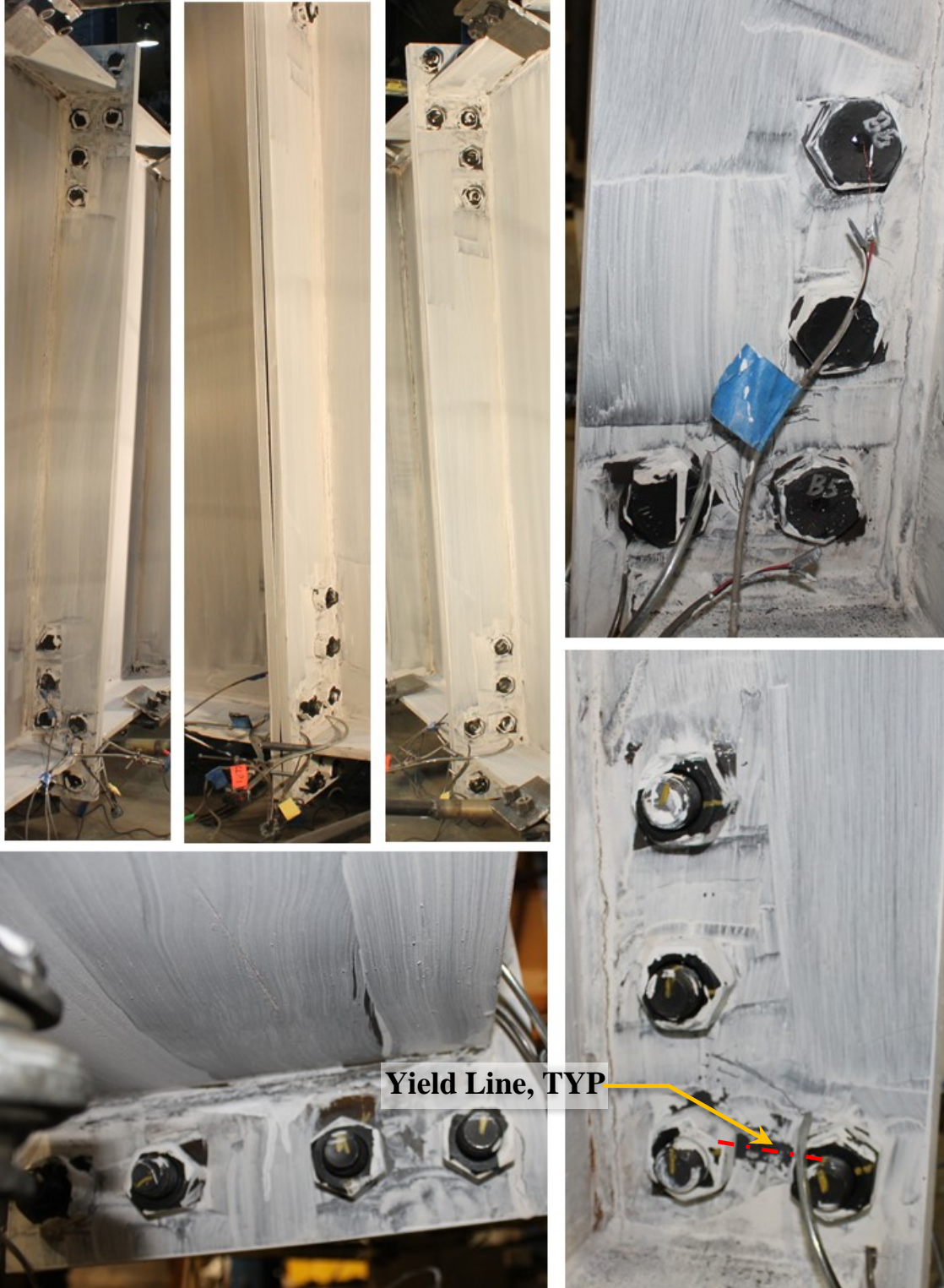
Figure 6-38 Three views of the specimen 12B-MRE 1/3-4W/2W-1.00-0.75-60 and zoomed in views of the connection to show any yield lines, at the end of the test
