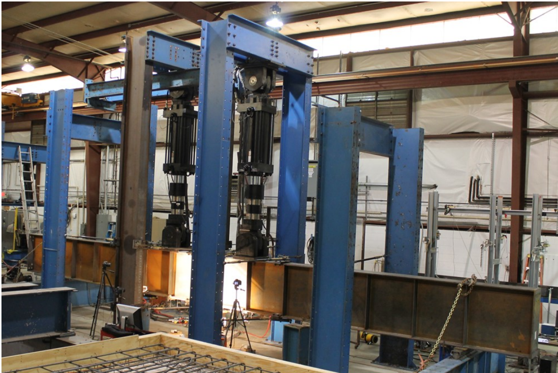
Figure 5-8 Picture of a Typical Shallow Beam Test Setup
