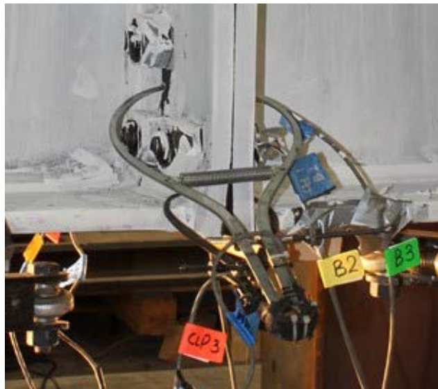
Figure 5-12 Instrumented Calipers Measuring End-Plate Separation
