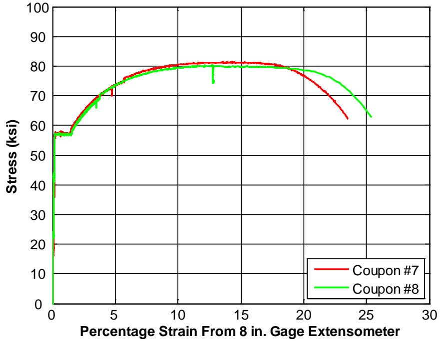
Figure 5-17 Results of Tensile Coupon Testing for 0.75 in. thick end-plate
