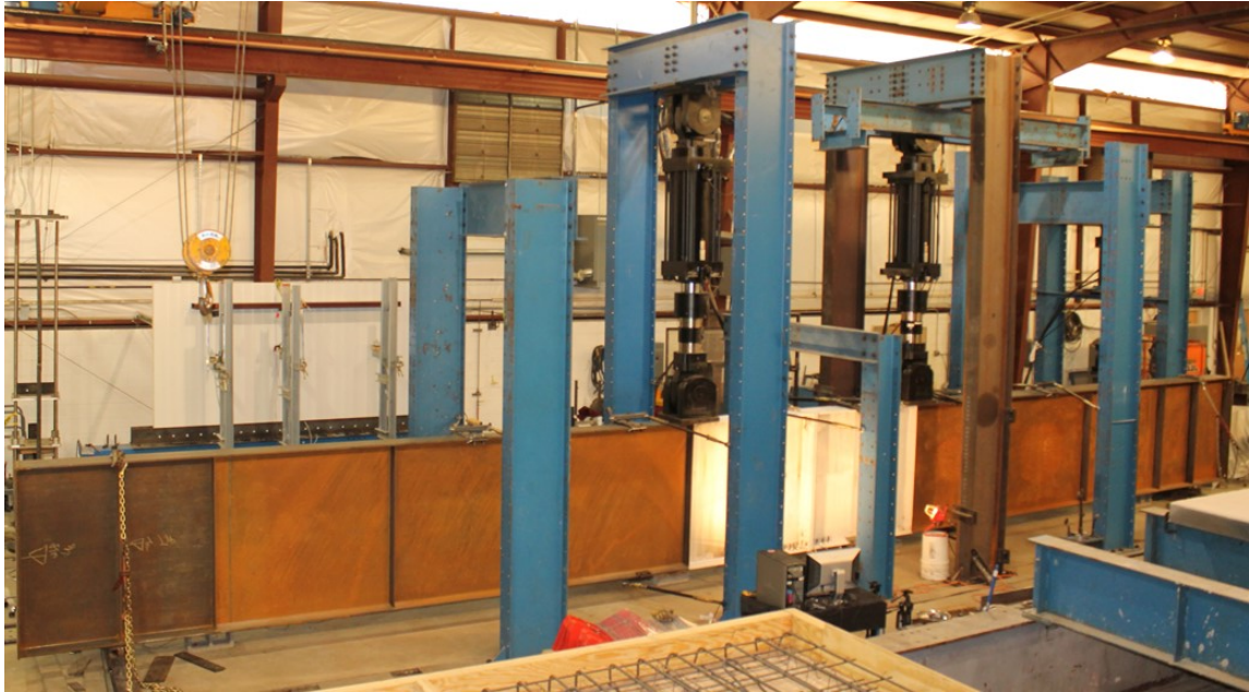
Figure 5-7 Picture of a Typical Deep Beam Test Setup
