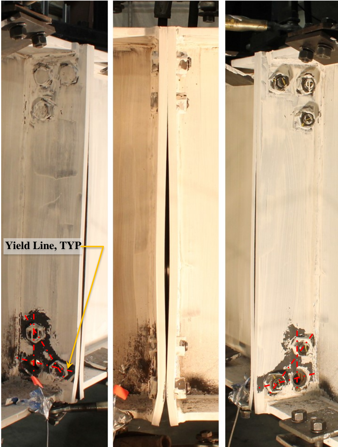
Figure 6-5 Three views of the specimen 6B-4W/2W-1.125-0.75-36 at the end of the test
