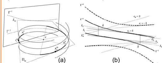
**Triple-source helical cone-beam tomography** formulated by Lv Y, Katsevich A, Zhao J, Yu H and Wang G (2010). (a) An intersection line of an osculation plane and the detector plane and (b) representative filtering lines.
