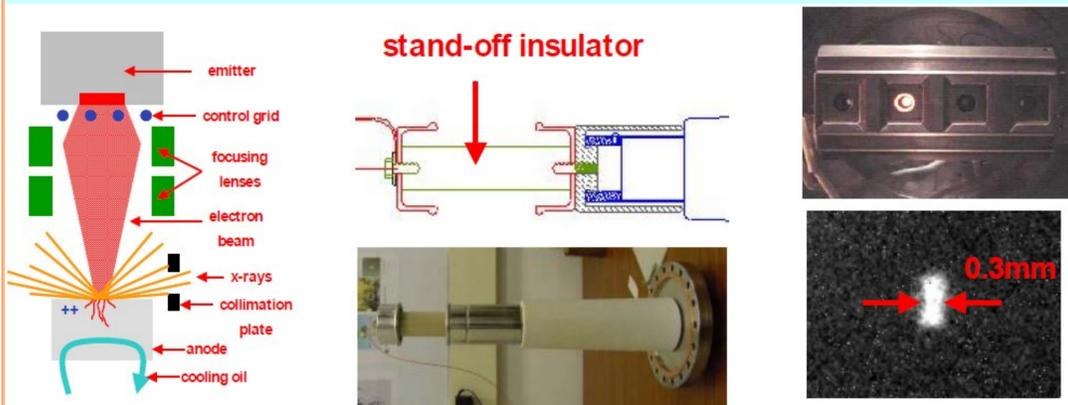
**Distributed x-ray source technology** developed by GE Global Research Center. (a) Diagram of a multi-source electron gun topology, (b) drawing and picture of a high-voltage standoff insulator, and (c) a fast-switching x-ray cathode with 4 focal spots, with measurement of a focal spot.
