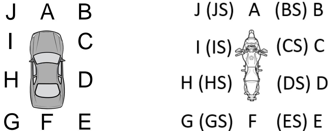
Figure 5. Regarding Motorist/Non-Motorist/Animal/Object Location. Subject vehicle is pictured. Location of conflicting vehicle, person, animal, or object is coded A-J in relation to subject vehicle. “S” is denoted for lane-sharing motorcycles. K is used for top of vehicle.
