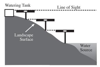
Figure 2. A method for measuring elevation changes.
