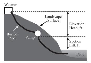
Figure 1. Suction lift and elevation head.
