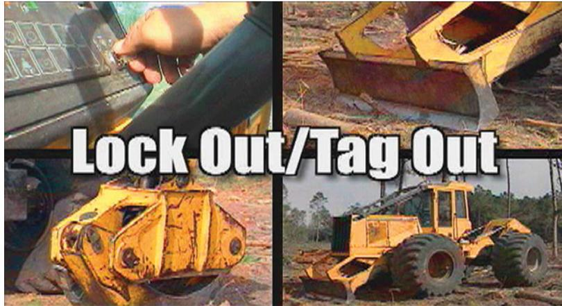
Next we'll cover the lockout-tagout procedures for maintaining or servicing the skidder. When maintenance is required on a skidder or other piece of machinery, lockout-tagout will help ensure the safety of the mechanic and others nearby.
