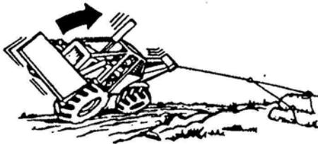
Winch load in straight line to avoid rollover.
