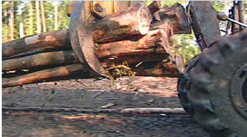
Maintain as level a position as possible, avoiding steep slopes. Never skid across the slope or at sharp angles.
