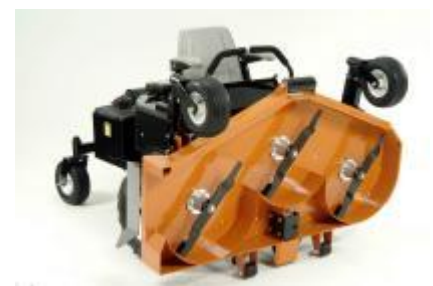
Decks are designed to chop grass clippings several times before discharge
