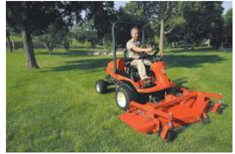
Ground carried deck
