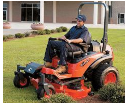
Suspended mower deck with parallel links
