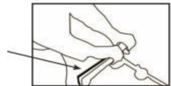
Note the "clutch-handle" that must be closed to keep engine running.
