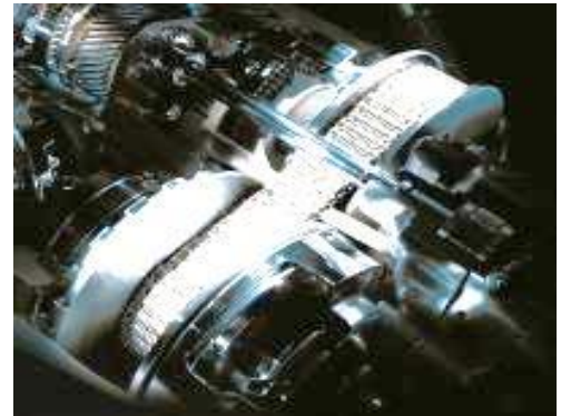
Belt and conical pulley system for continuously varying the speed.
