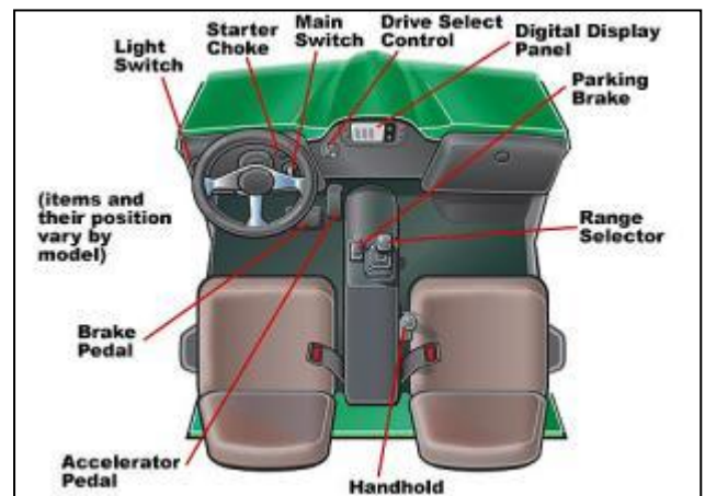
Operator's controls platform.
