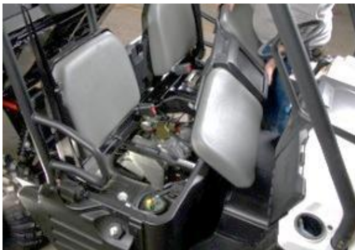
Liquid cooled engine - radiator under the seat.
