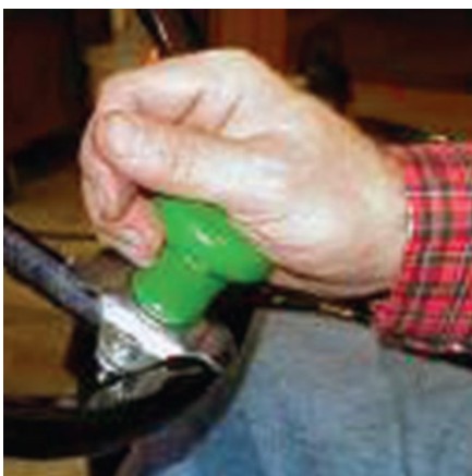
Figure 4. Steering wheel with a spinner knob for ease of moving the steering wheel.
