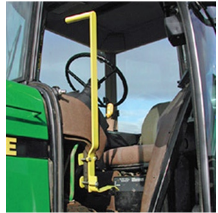
Figure 3. Hand-control linkage for operating the clutch.
