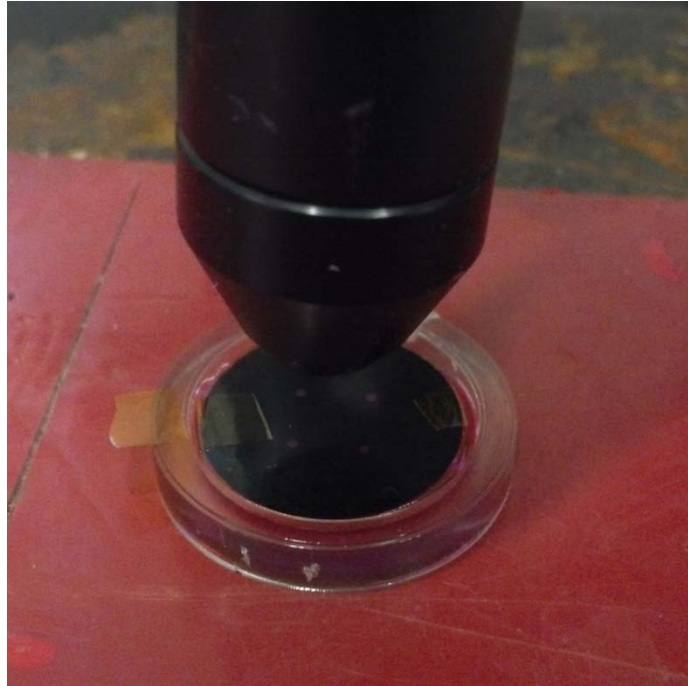
Figure 2-7. Hydrogels in the process of curing for a 2x2 array. A printed mask over a glass slide covers the liquid hydrogel on the substrate.
