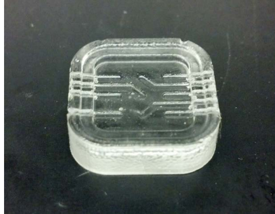
Figure 3-22. Base substrate for 3x3 array after removal from the mold.
