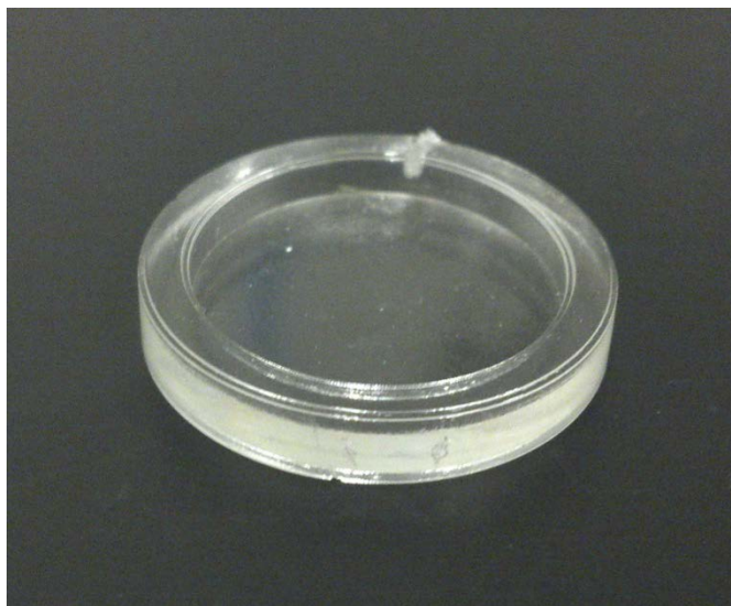
Figure 2-5. Circular polyurethane substrate designed to contain oil phase used in bilayer experiments.
