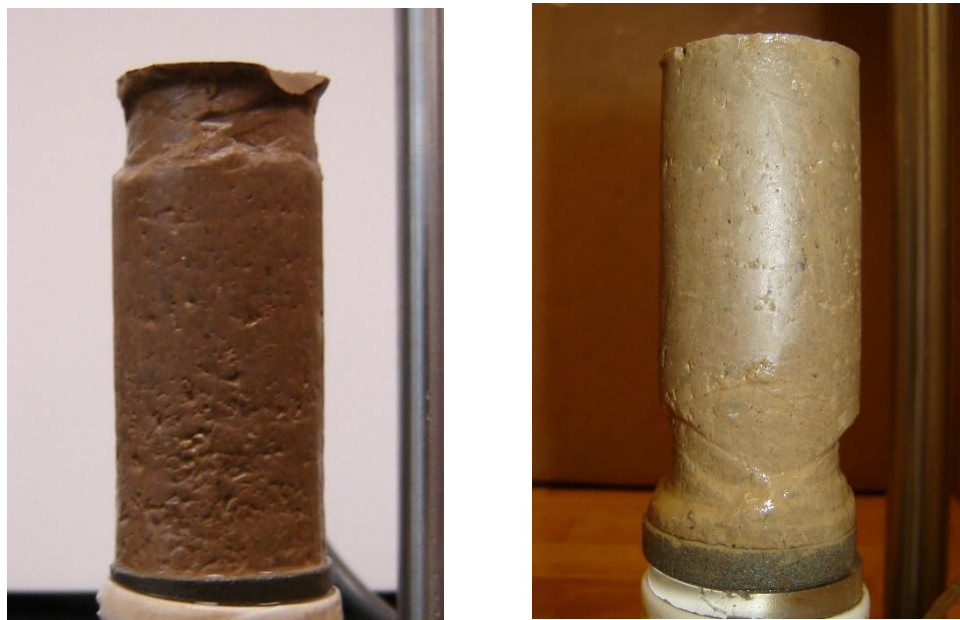
Figure 3-13. Necking in two TE specimens of compacted Oak Harbor clay
