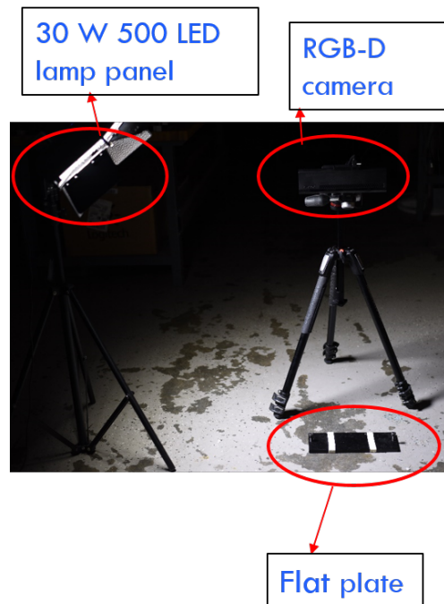
Figure 4.3: Precision of depth values experimental setup
