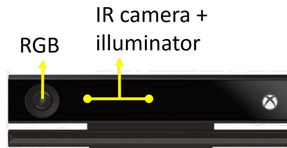
(a) Kinect v2's components
