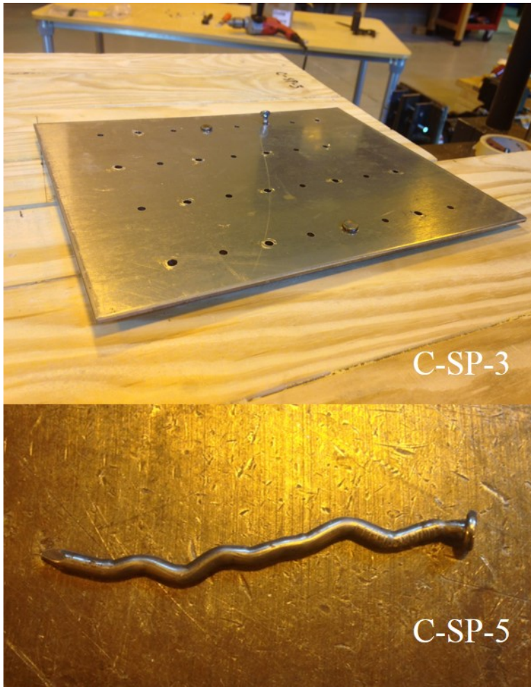
Figure 4-29: Photographs of Fastener Withdrawal from Steel Plate Specimens
