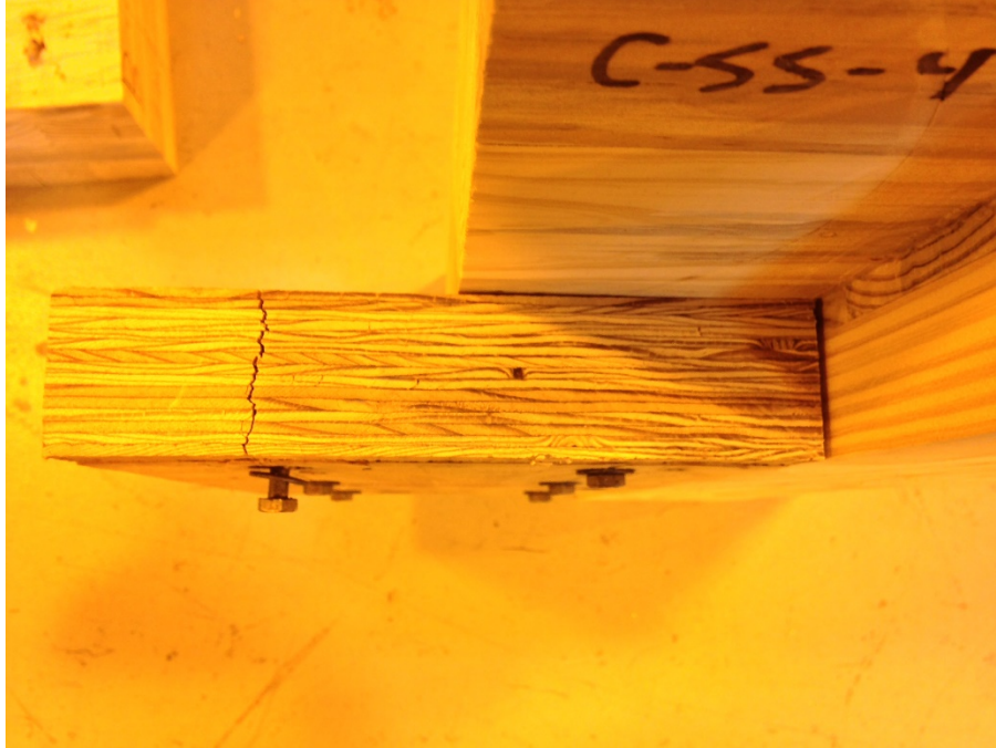
Figure 4-25: Partial Shear Parallel to Grain Failure in LVL Spline for C-SS-4
