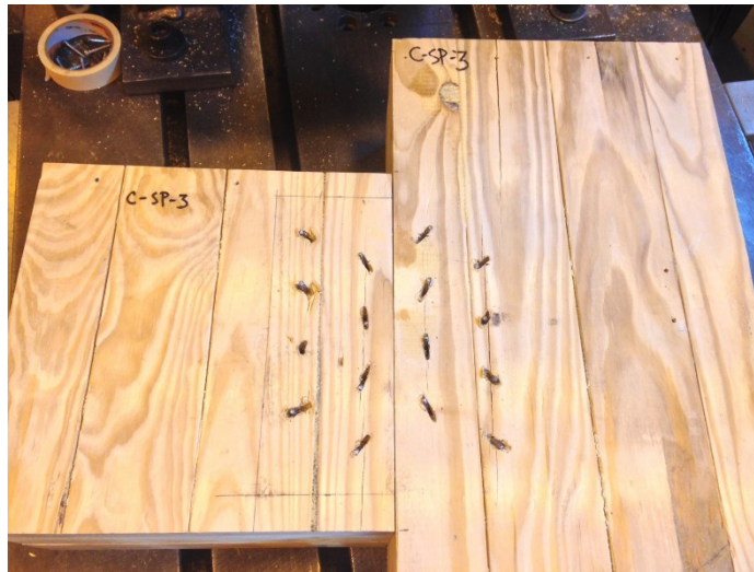
Figure 4-27: Photograph of Diagonal Wood Crush Caused by Plate Rotation
