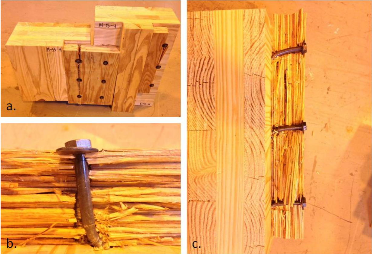
Figure 4-10: Photographs of LVL Spline Failure in M-SS-4
