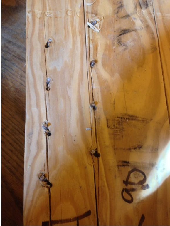
Figure 4-15: Photograph of Splitting Due to Shear Parallel to Grain in M-SP-2
