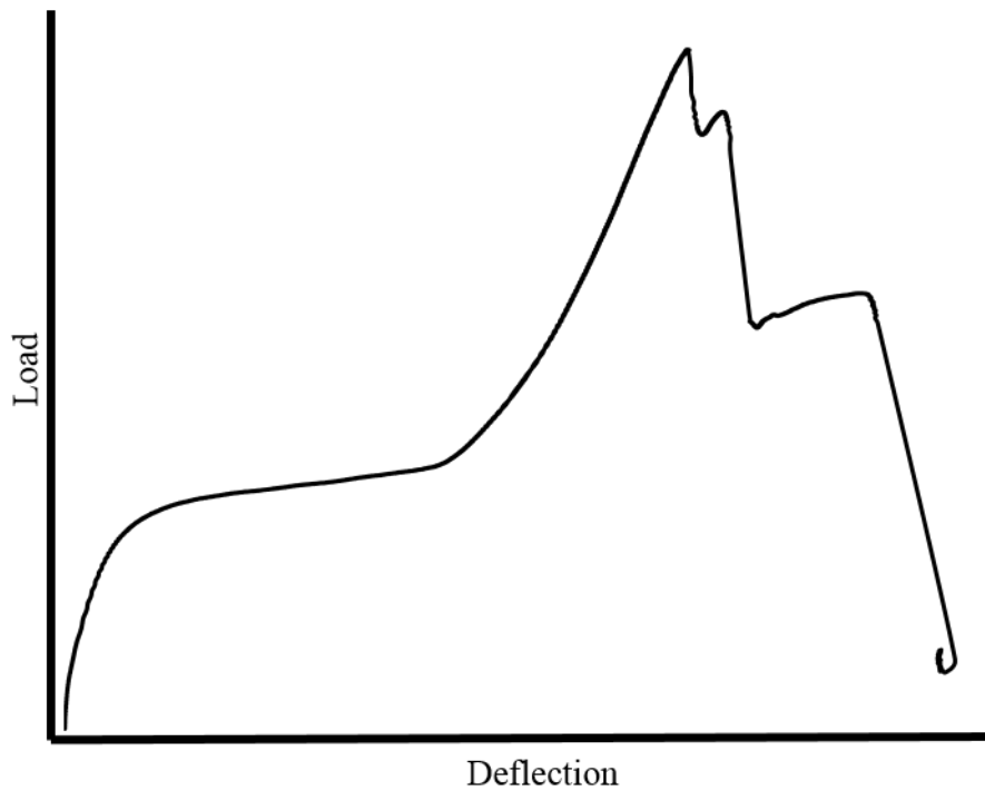
Figure 4-3: Load-Deformation Curve for a Half-Lap Specimen
