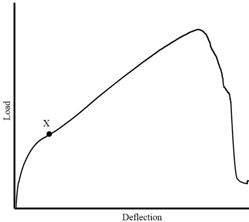
Figure 4-2: Load-Deformation Curve for a Surface Spline Specimen
