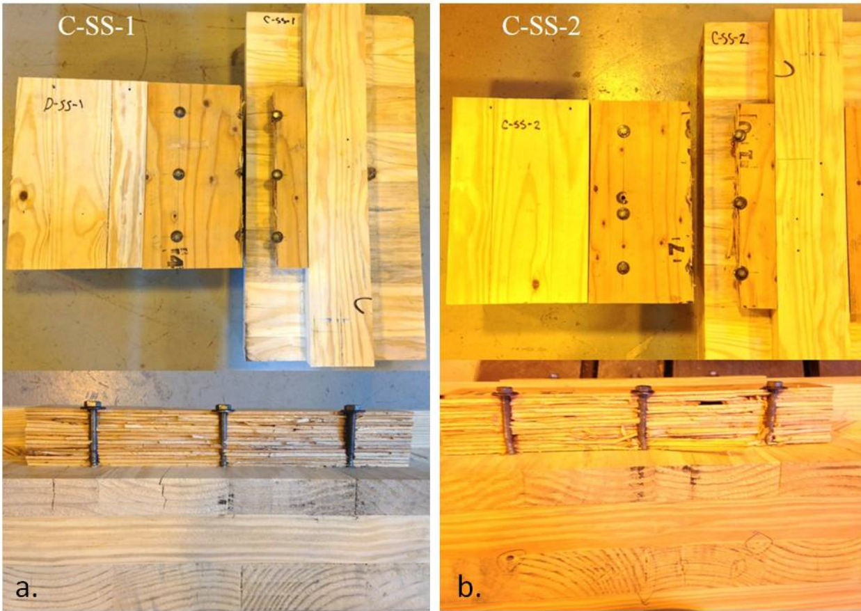
Figure 4-23: Photographs of Damages from Specimens C-SS-1 and C-SS-2
