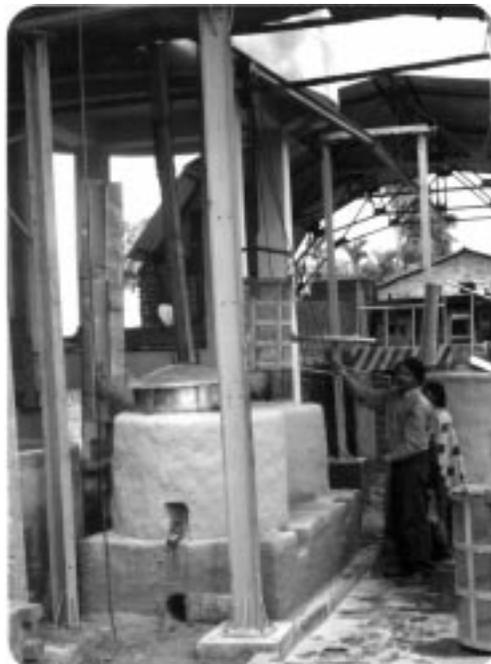
*Low-tech papermaking equipment. Haridash demonstrates hoisting digested pulp from his new efficient woodstove (lower left) using his new overhead trolley system.*
