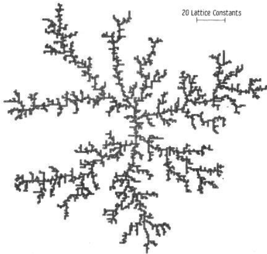
Figure 2.8: Random aggregate of 3600 particles on a square lattice [Witten, T. A and L. M. Sander, “Diffusion-Limited Aggregation, a Kinetic Critical Phenomenon” The American Physical Society , Vol 47 No 19, 1981.] Used under fair use, 2015.
