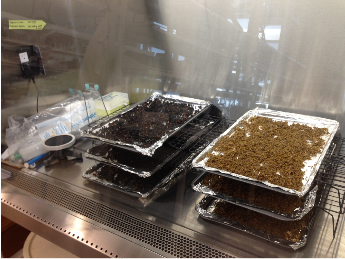
Figure 4.1: Drying set up for inoculated seeds. Inoculated seeds were spread in a thin, single layer on foil-lined metal baking sheets suspended on cooling racks and allowed to dry for 24 hours in a BSL2 continuous air-flow hood to achieve 0.30 water activity.
