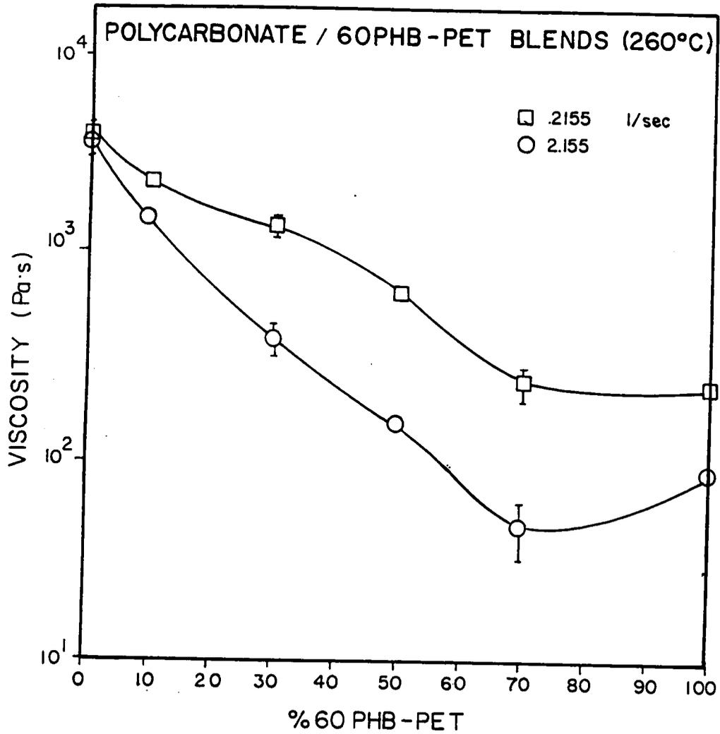
Figure 4.14. Steady shear viscosity of PC blends as a function of composition for two shear rates in the RMS.
