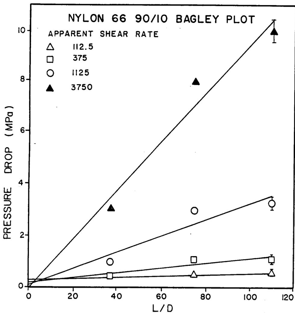
Figure B.7. Bagley Plot for 90/10 N66/LCP at 275°C.
