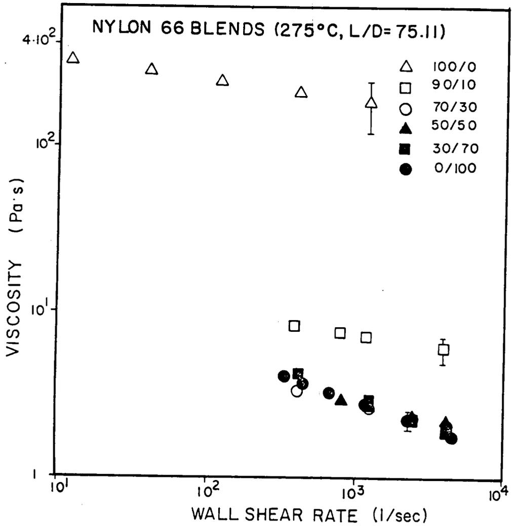
Figure 4.23. Viscosity of N66 blends from the ICR.
