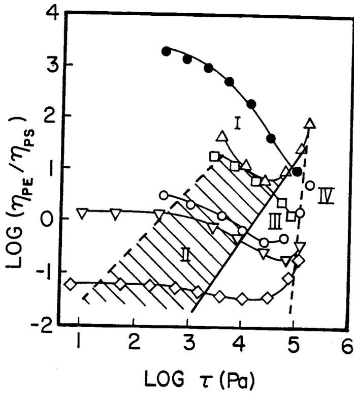
Figure 2.1. Viscosity ratio versus shear stress for PE in PS blends. Region I, no fibers; II, imperfect fibers; III, perfect PE fibers; IV, disintegrated fibers. From [26].
