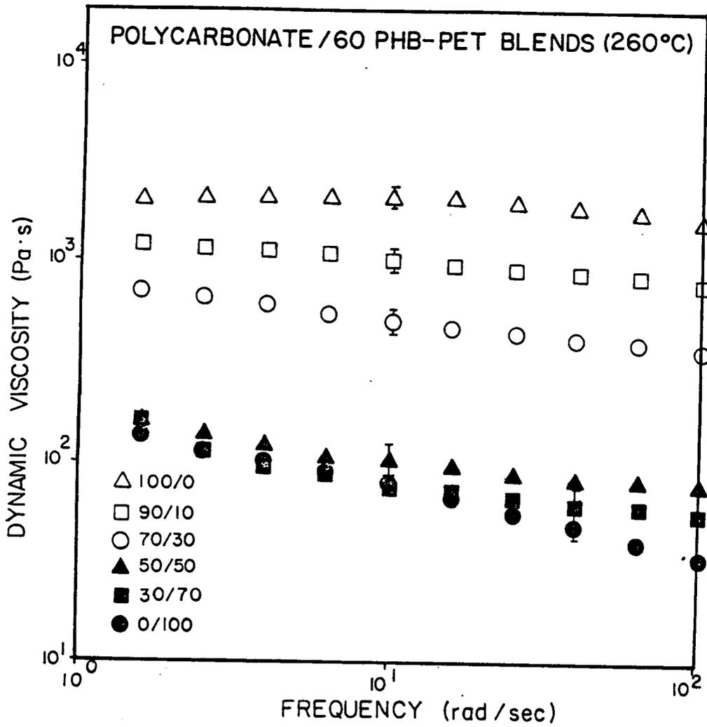
Figure 4.15. Dynamic viscosity of PC blends from the RMS.
