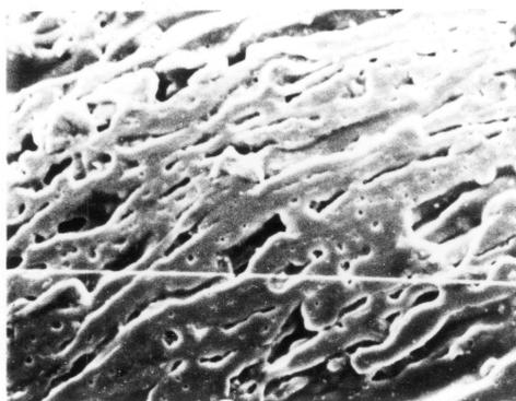
Figure 4.4. Micrographs of extruded N66 blends after extraction of N66. a, 30% LCP; b, 50% LCP; c, 70% LCP. 480 x.
