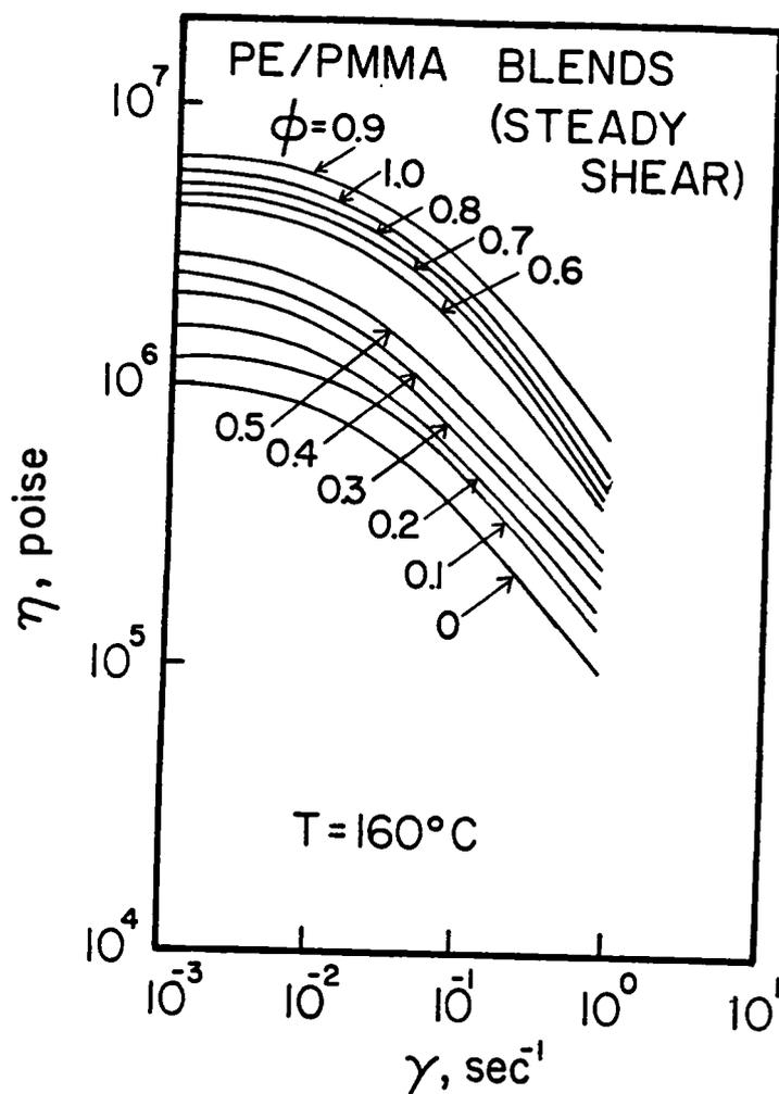
Figure 2.9. Smoothed curves for non-Newtonian viscosity for PE/PMMA blends. From [48].
