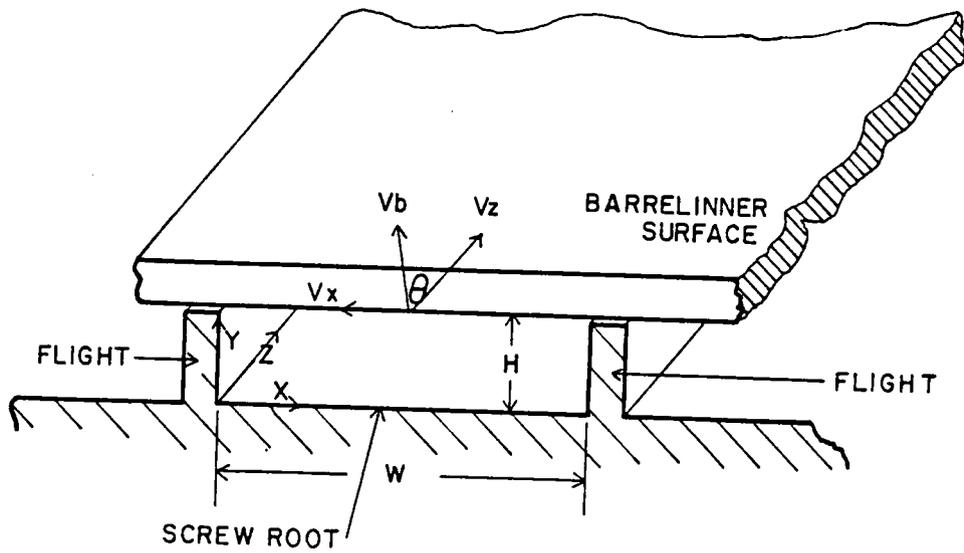
Figure 2.17. Rectangular representation of the flow channel in single screw extruders. From [76].
