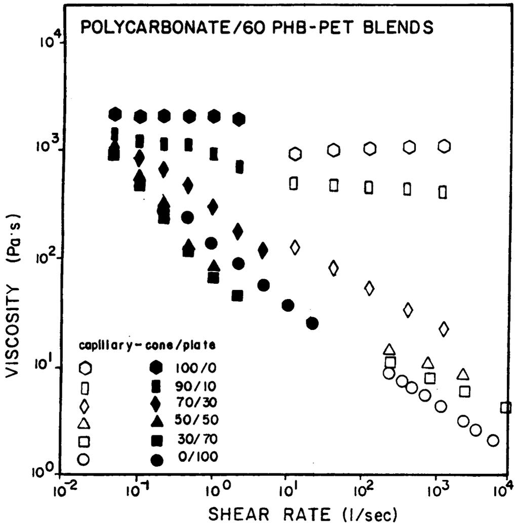
Figure 4.22. Combined viscosity data from RMS and ICR for PC blends.
