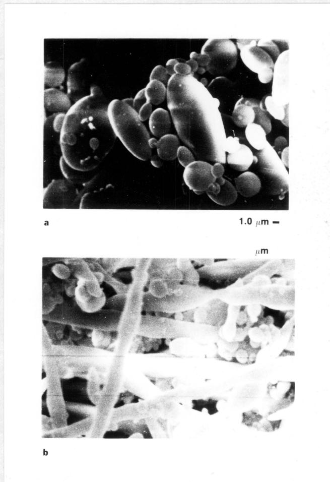
Figure 4.2. Micrographs of extruded PC blends after extraction of PC. a, 10% LCP; b, 30% LCP. 4000 x.
