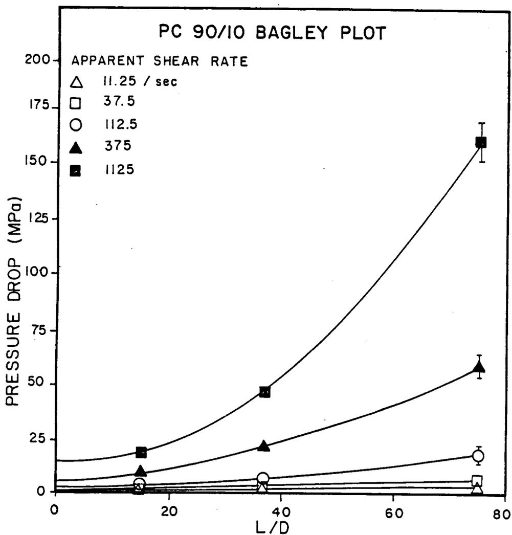
Figure B.2. Bagley Plot for 90/10 PC/LCP at 260°C.
