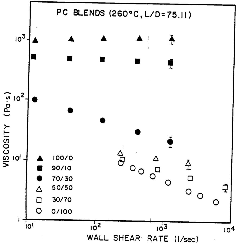
Figure 4.20. Viscosity of PC blends from the ICR for an L/D of 75.11 and a capillary diameter of 0.0686 cm.
