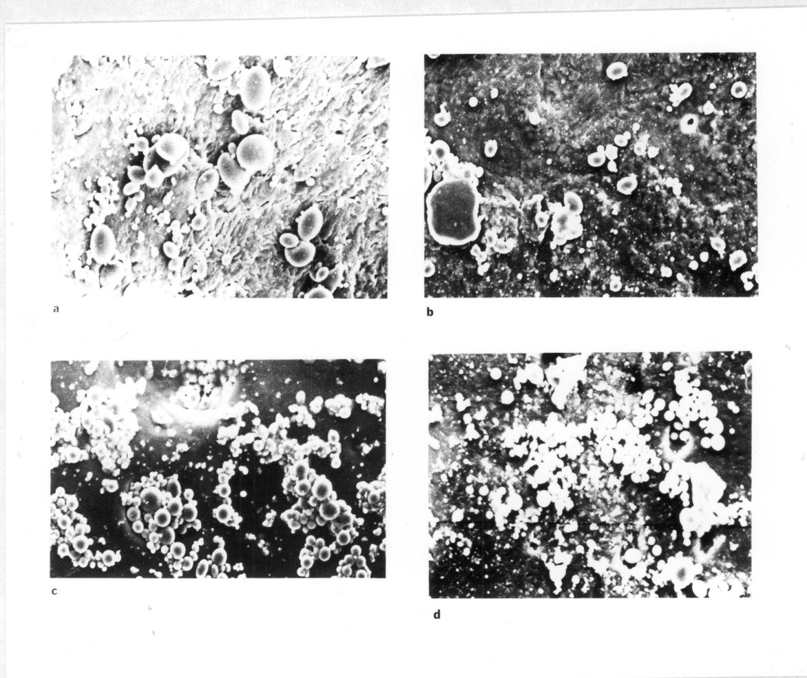
Figure 4.7. Micrographs of 30% LCP after extraction of PC for increasing shear rates. a, 0.1/sec; b, 1.0/sec; c, 10/sec; d, 100/sec. 480 x (except c which is 940 x).
