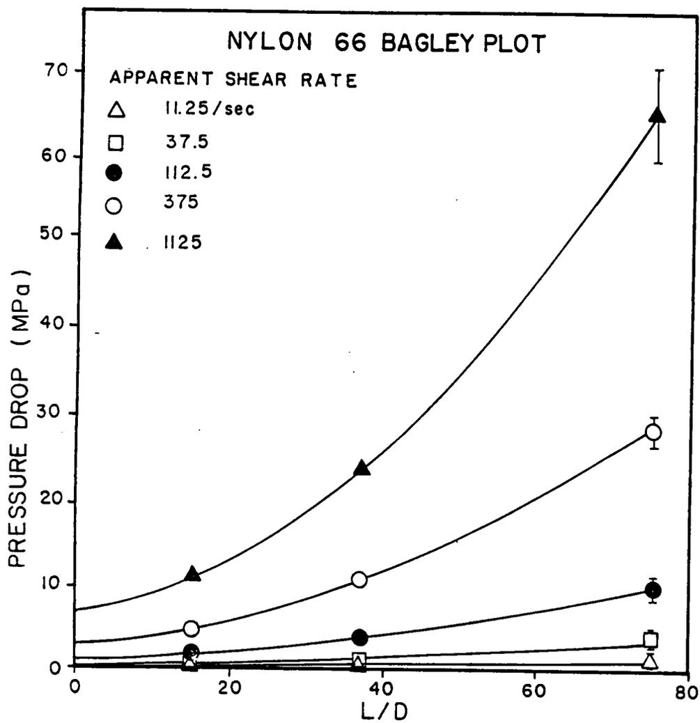
Figure B.6. Bagley Plot for Nylon 6,6 at 275°C.
