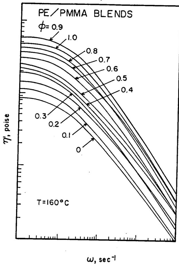
Figure 2.8. Smoothed curves for dynamic viscosity of PE/PMMA blends, for all volume fractions. From [48].
