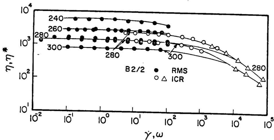
Figure 2.13. Viscosity of 10% PA 6,6 in PET at four temperatures for both RMS and ICR measurements. From [41].
