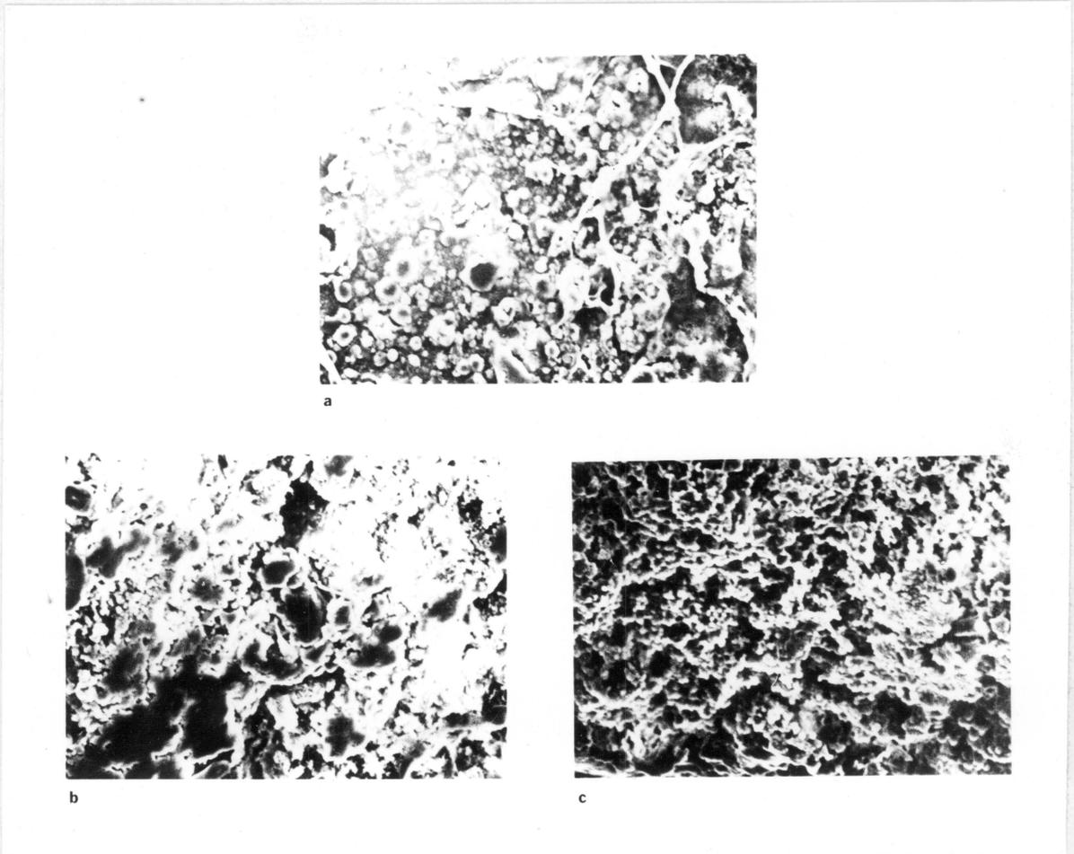
Figure 4.9. Micrographs of 30% LCP after deformation in RMS and extraction of N66. a, no shear; b, 10/sec; c, 100/sec. 480 x.
