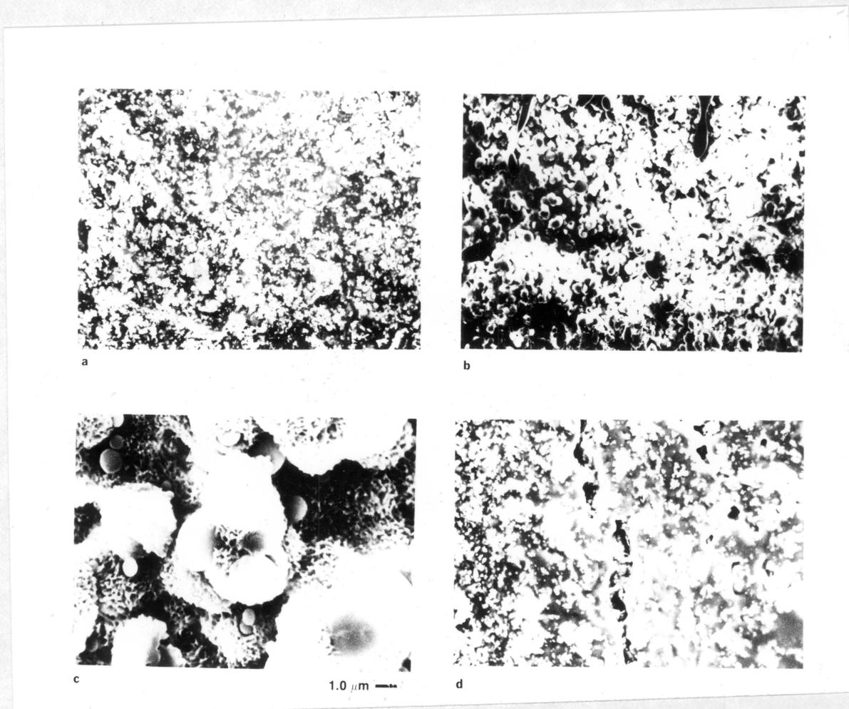
Figure 4.11. Micrographs of 30% LCP after extraction of PC. Samples extruded through ICR with L/D of 21.4. a, 45.7/sec; b, 137/sec; c, 137/sec at 4800 x; d, 457/sec. a, b, and d at 480 x.
