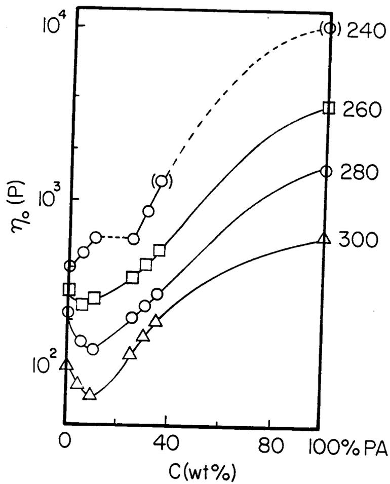
Figure 2.12. Compositional dependence of zero shear viscosity at four temperatures for PET/PA 6,6 blends. From [41].
