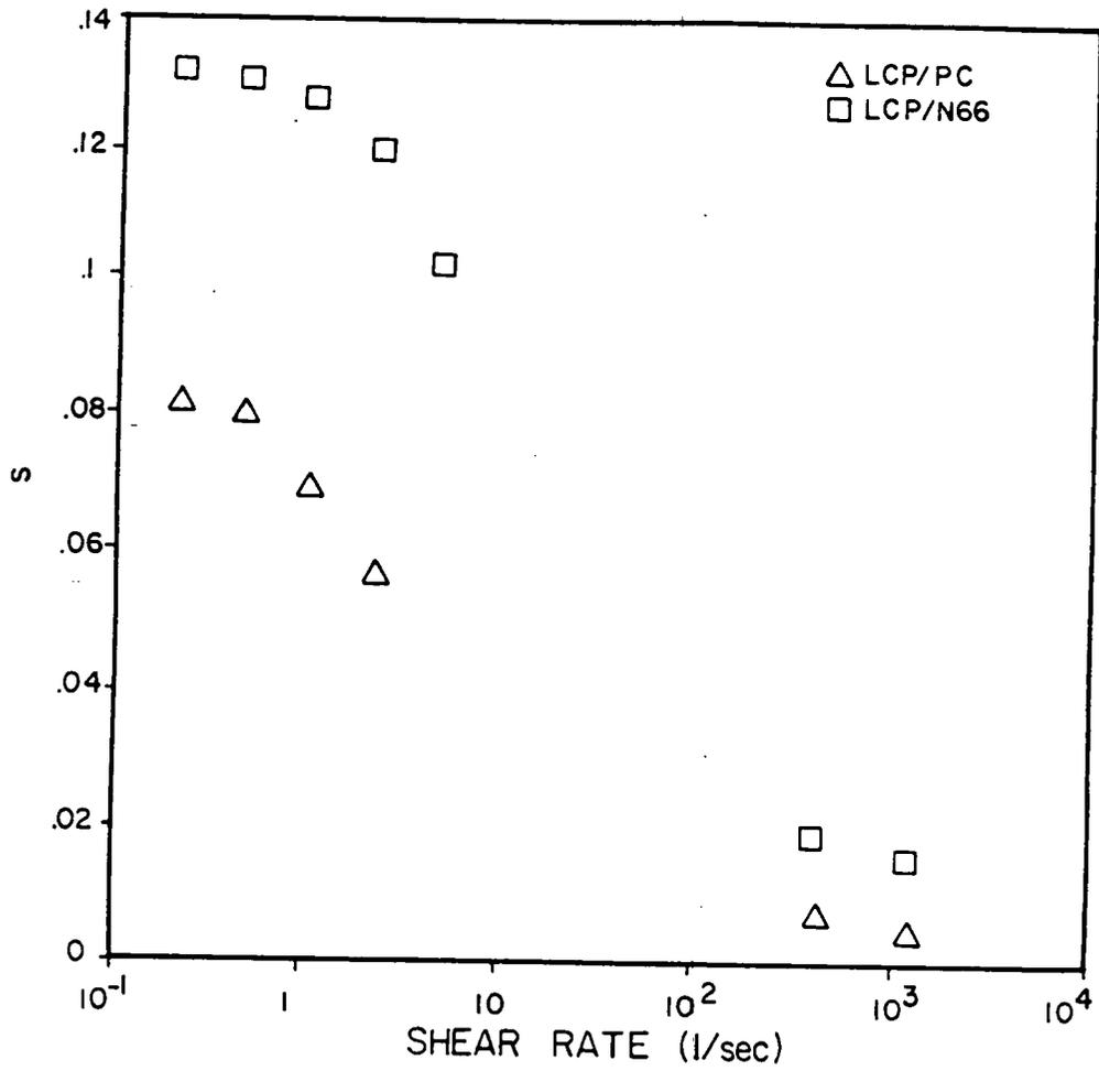
Figure 4.26. Viscosity ratio of LCP to thermoplastic for the shear rates studied in the RMS and ICR.
