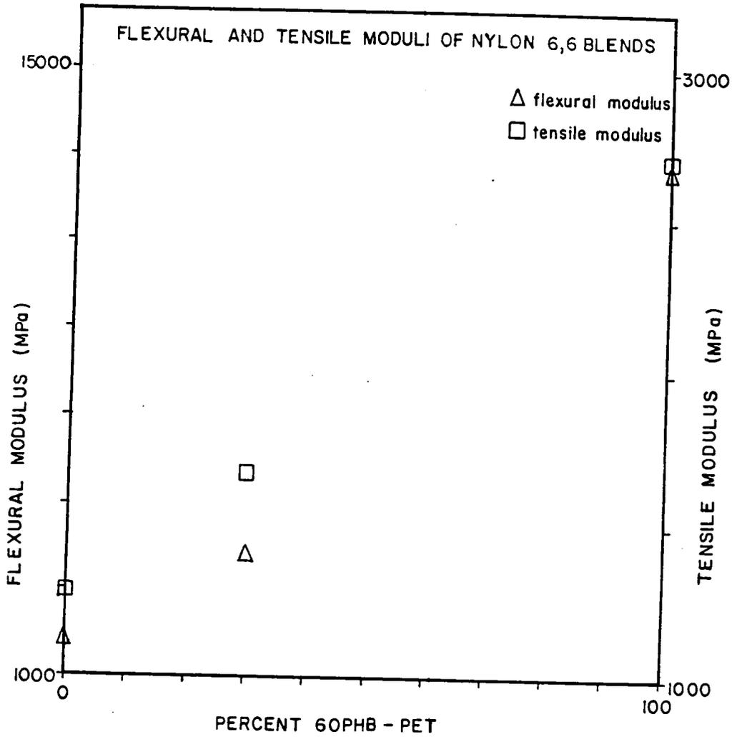
Figure 4.28. Flexural and Tensile Moduli of N66 blends. Values taken at 35% relative humidity and 26°C along the flow direction.
