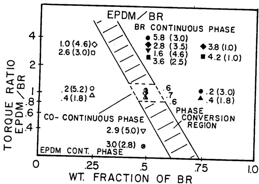
Figure 2.3. Morphology changes as a function of torque ratio and composition. Numbers represent domain diameter in  $\mu\text{m}$  and length to diameter ratio in parentheses. Shaded symbols indicate EPDM as dispersed phase, open symbol BR. From [33].
