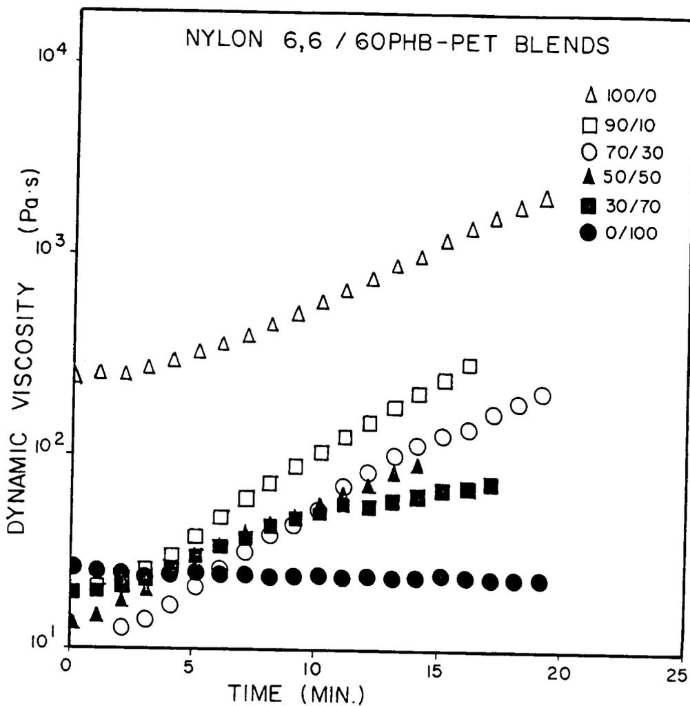
Figure 3.3. Dynamic time sweep of N66 blends at 275°C and 10 sec<sup>-1</sup> for an unbaffled system.
