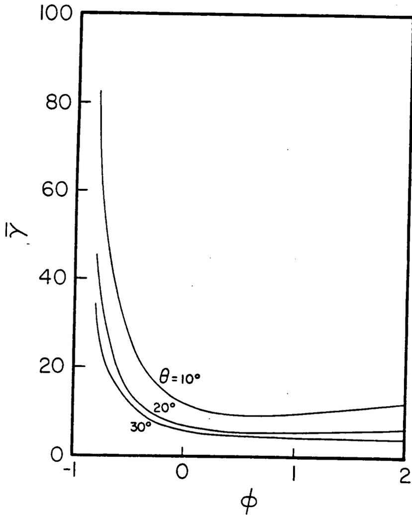
Figure 2.18. The weighted average total strain as a function of  $\phi$  at various helix angles. From [76].
