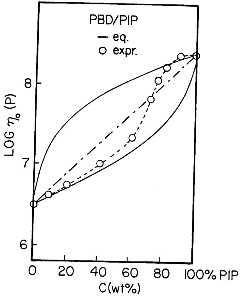
Figure 2.6. Viscosity of PBD/PIP blends as a function of concentration. From [46].
