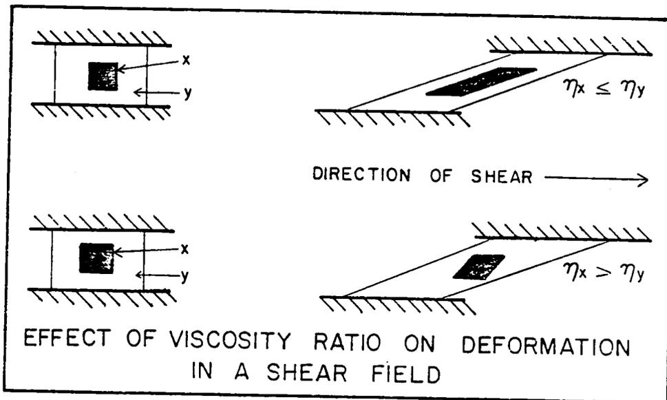
Figure 2.15. The effect of viscosity ratio of the minor to major component on the deformation in a simple shear field.
