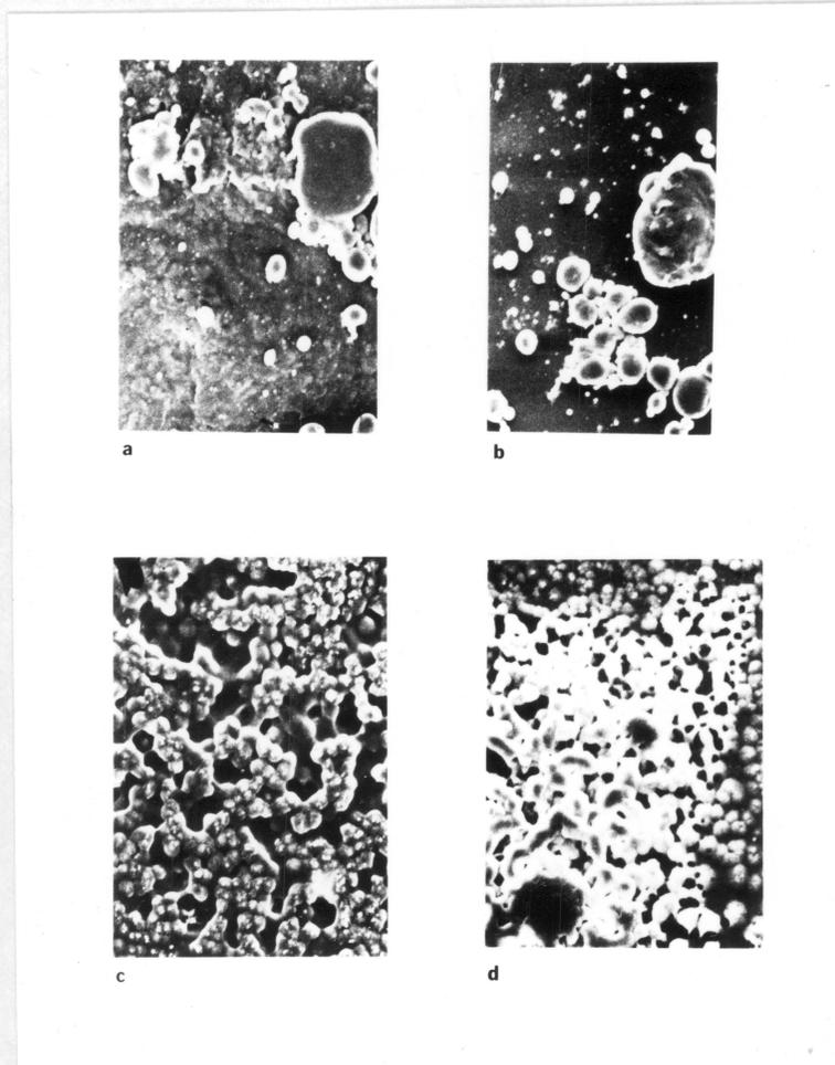
Figure 4.8. Micrographs of 30% LCP after deformation in RMS and extraction of PC. a, strain of 30 at 1/sec; b, strain of 100 at 1/sec; c, strain of 100 at 10/sec; d, strain of 5000 at 10/sec. 480 x.
