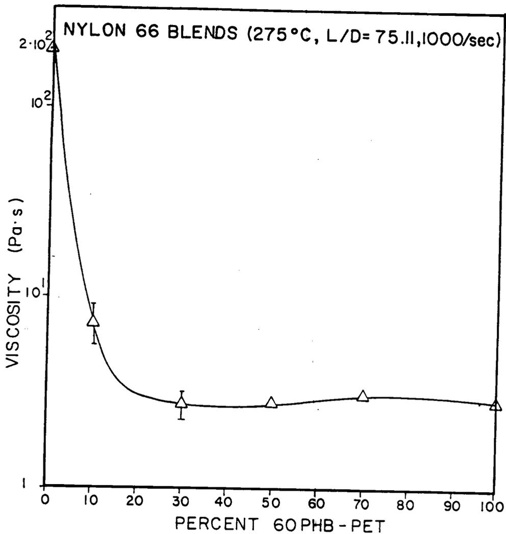
Figure 4.24. Viscosity of N66 blends at 1000/sec as a function of composition from the ICR.
