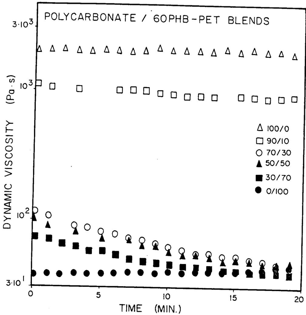
Figure 3.5. Dynamic time sweep of PC blends at 260°C and 10 sec<sup>-1</sup>.
