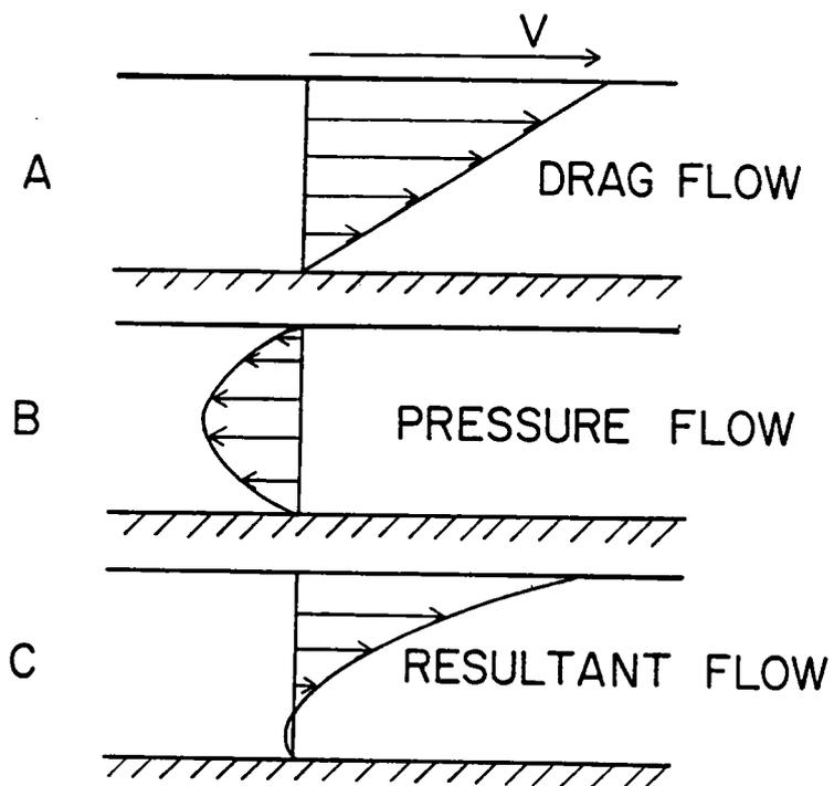
Figure 2.16. The velocity profile for a Newtonian fluid in parallel plate geometry. From [74].
