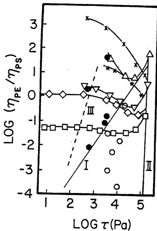
Figure 2.2. Viscosity ratio versus  $\tau$  for PE/PS mixtures. Open circles represent fibril formation in a rotary viscometer, closed circles show no fibril formation. Other symbols from capillary results (Fig. 2.1). From [27].
