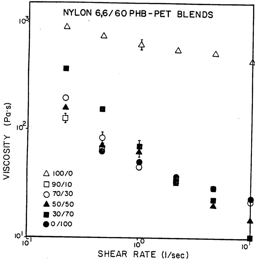
Figure 4.17. Steady shear viscosity of N66 blends from RMS. The first number appearing in the key denotes the weight percent of N66, the second that of the LCP.
