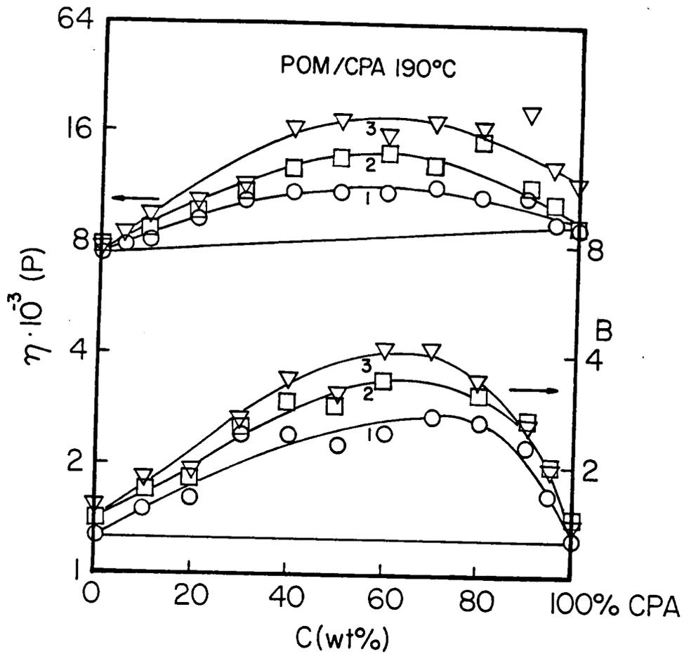
Figure 2.4. Viscosity and die swell of POM/copolyamide blend as a function of concentration. Number of times the sample was extruded is indicated. From [43].
