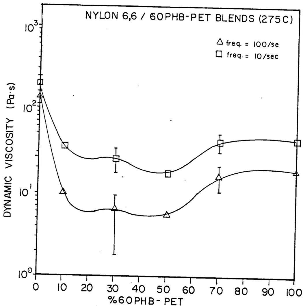
Figure 4.19. Viscosity of N66 blends as a function of composition for two shear rates from the RMS.
