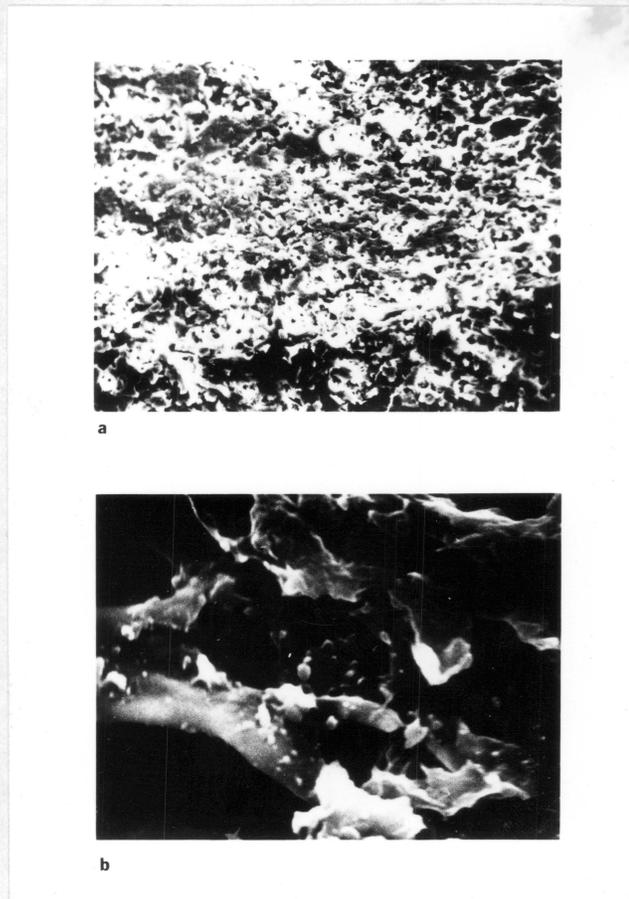
Figure 4.29. Micrographs of injection molded samples of 30% LCP after extraction of PC. Top surface of plaque at a, 480 x; b, 4800 x.
