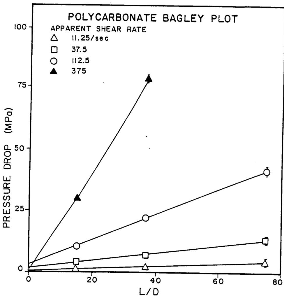
Figure B.1. Bagley Plot for Polycarbonate at 260°C.
