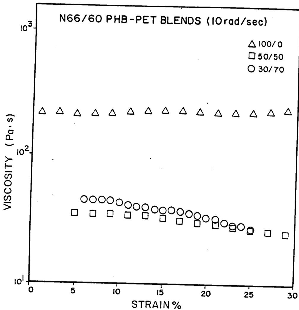
Figure 3.1. Dynamic strain sweep of N66 blends at 275°C and 10 sec<sup>-1</sup>. Cone/plate mode on RMS.
