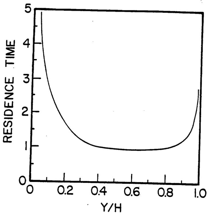
Figure 2.20. Relative residence time as a function of initial position in a single screw extruder. From [79].
