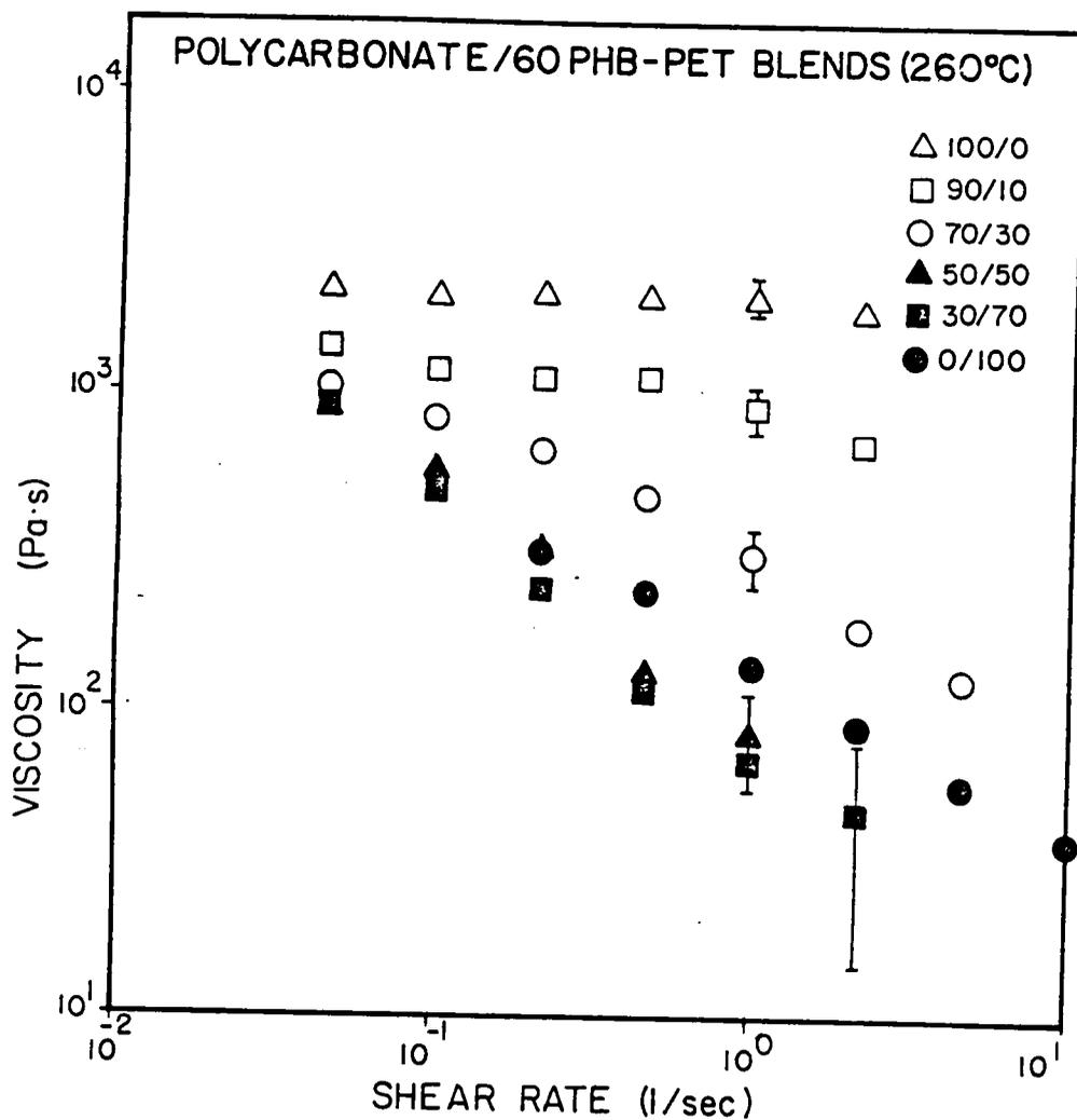
Figure 4.13. Steady shear viscosity of polycarbonate blends from RMS in cone & plate mode. The first number appearing in the key denotes the weight fraction of PC, the second that of the LCP.
