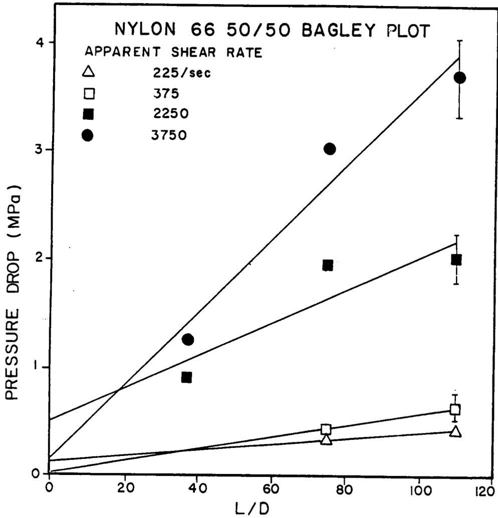
Figure B.9. Bagley Plot for 50/50 N66/LCP at 275°C.
