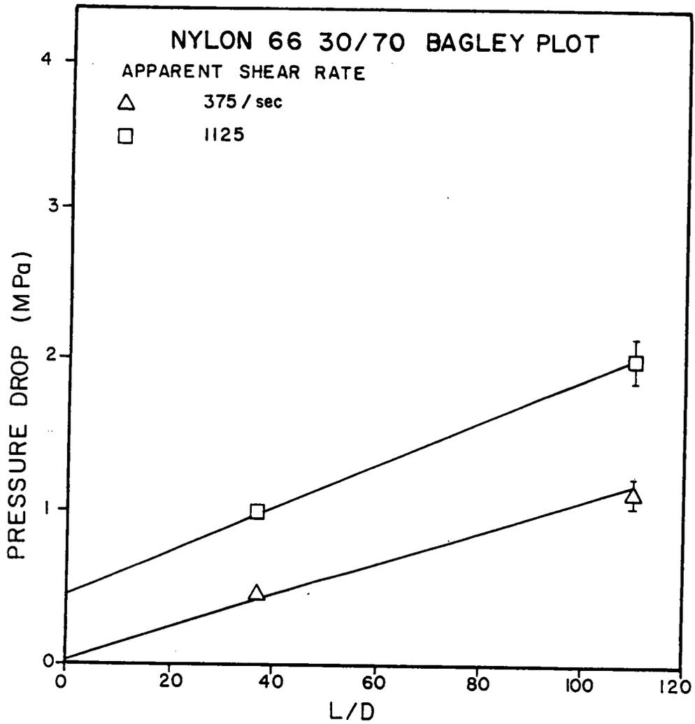
Figure B.10. Bagley Plot for 30/70 N66/LCP at 275°C.
