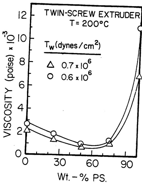
Figure 2.7. Viscosity versus blending ratio for PS/PP blends prepared with a twin screw extruder. From [25].
