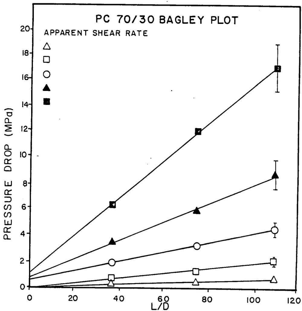
Figure B.3. Bagley Plot for 70/30 PC/LCP at 260°C.
