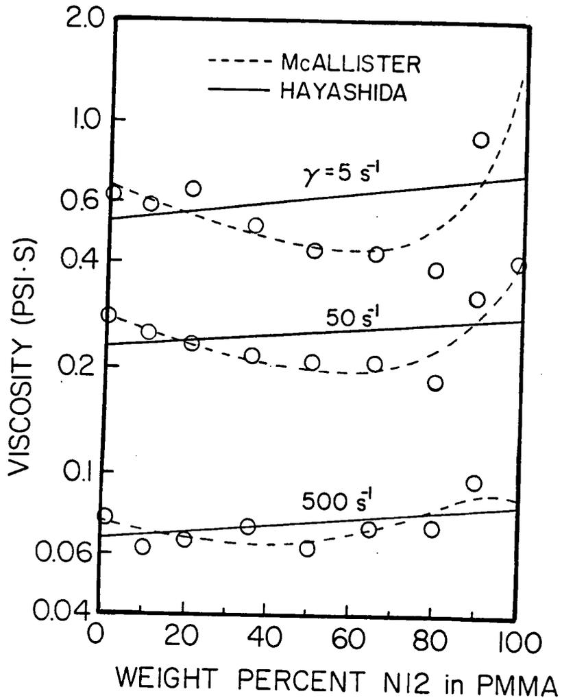
Figure 2.11. Viscosity dependence on composition for the N12/PMMA system. From [53].
