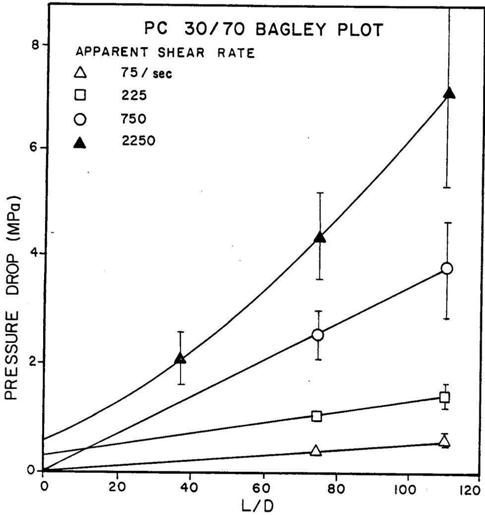
Figure B.5. Bagley Plot for 30/70 PC/LCP at 260°C.
