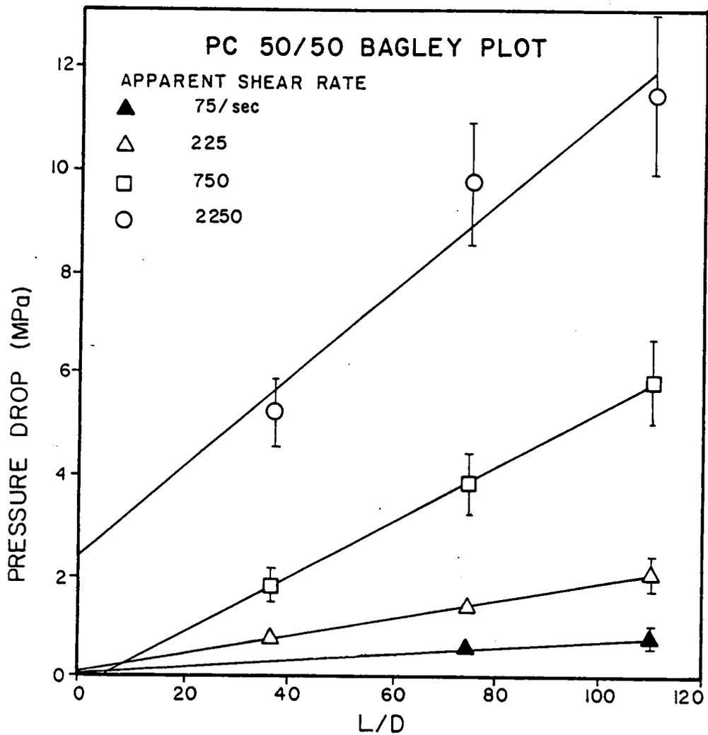
Figure B.4. Bagley Plot for 50/50 PC/LCP at 260°C.
