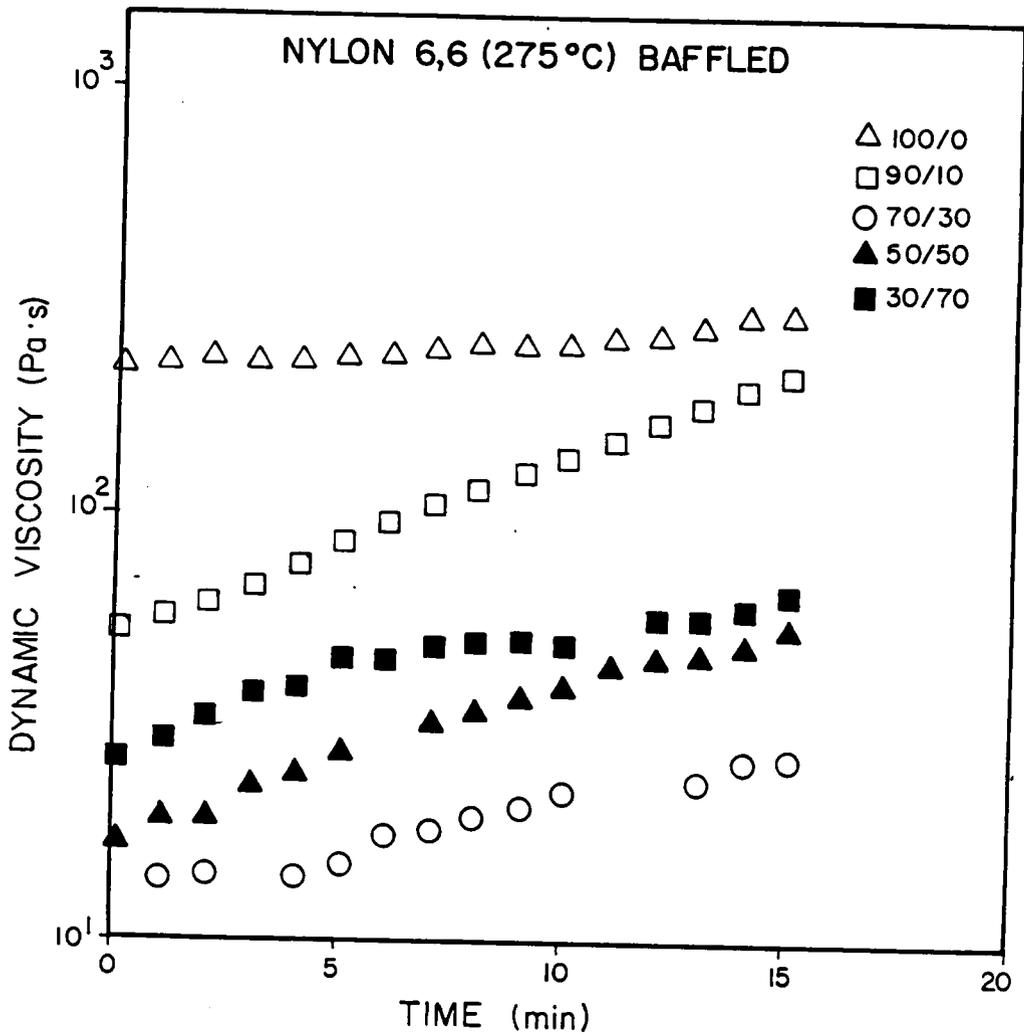
Figure 3.4. Dynamic time sweep of N66 blends at 275°C and 10 sec<sup>-1</sup> for the baffled system.
