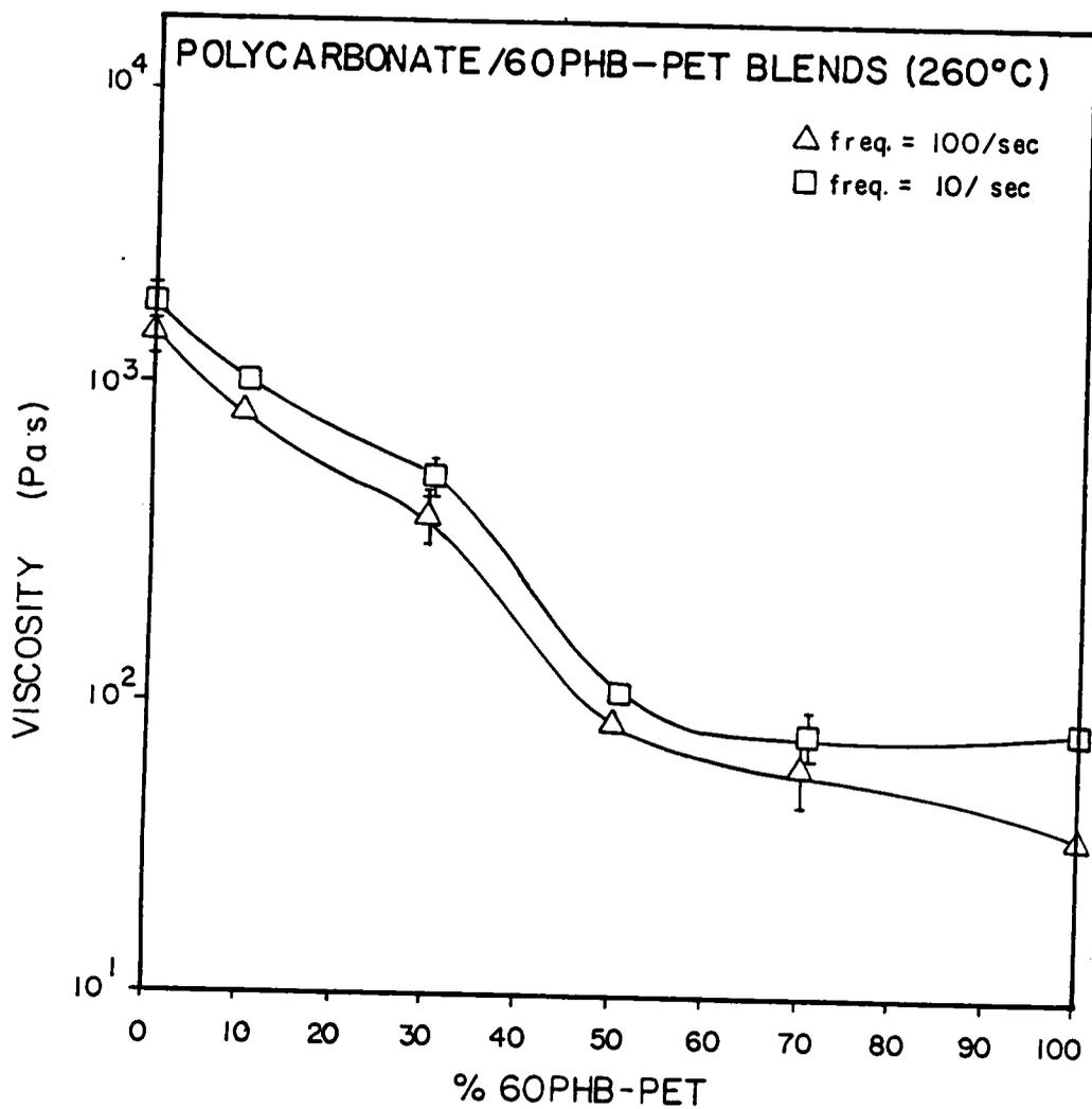
Figure 4.16. Dynamic viscosity of PC blends as a function of composition at two shear rates from the RMS.
