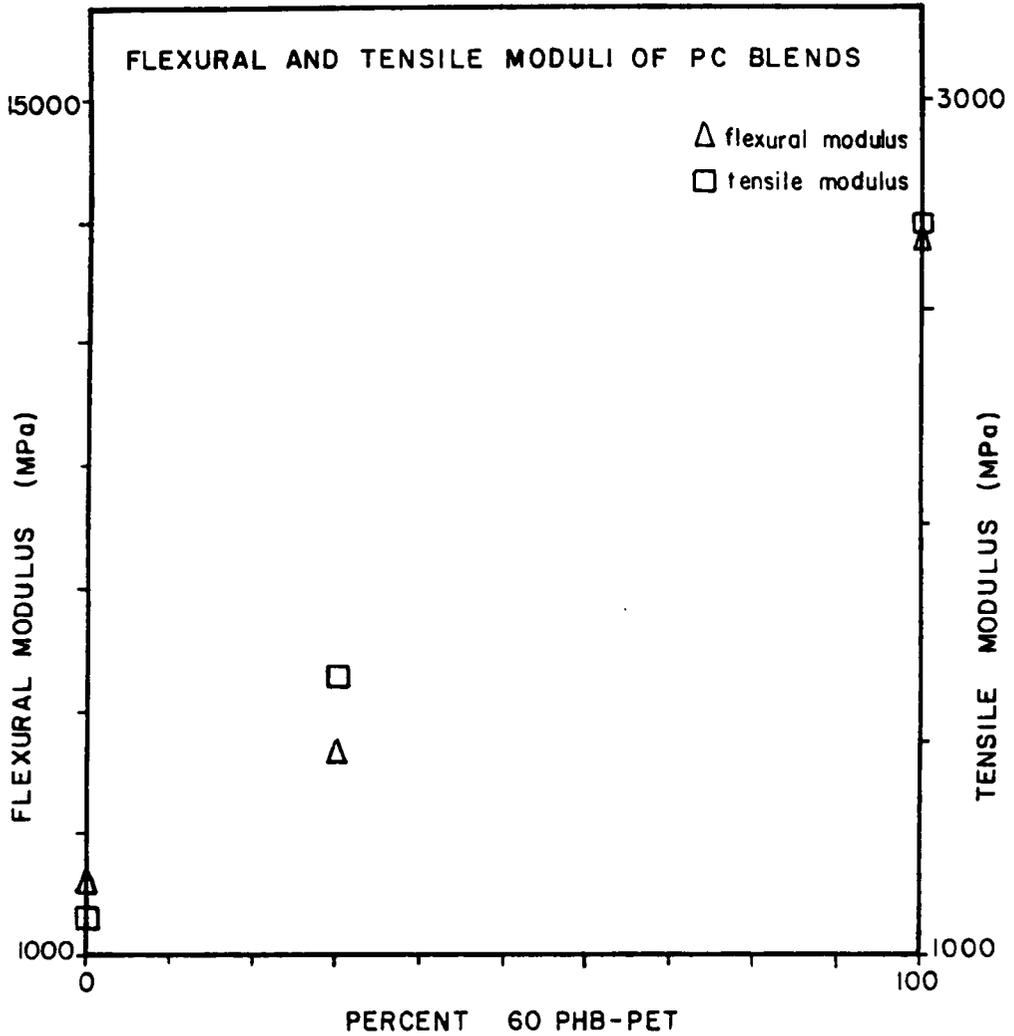
Figure 4.27. Flexural and Tensile Moduli of PC blends. Values taken at 35% humidity and 26°C along the flow direction.
