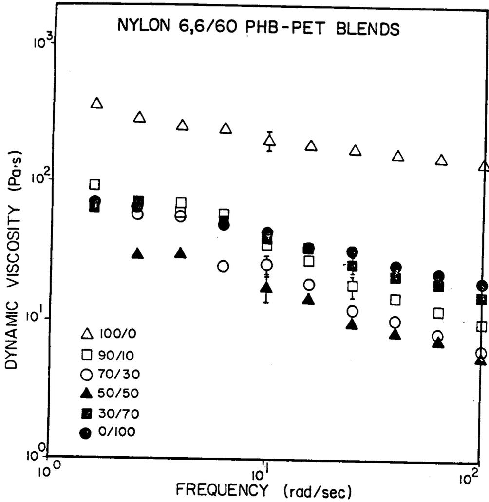
Figure 4.18. Dynamic viscosity of N66 blends from the RMS.
