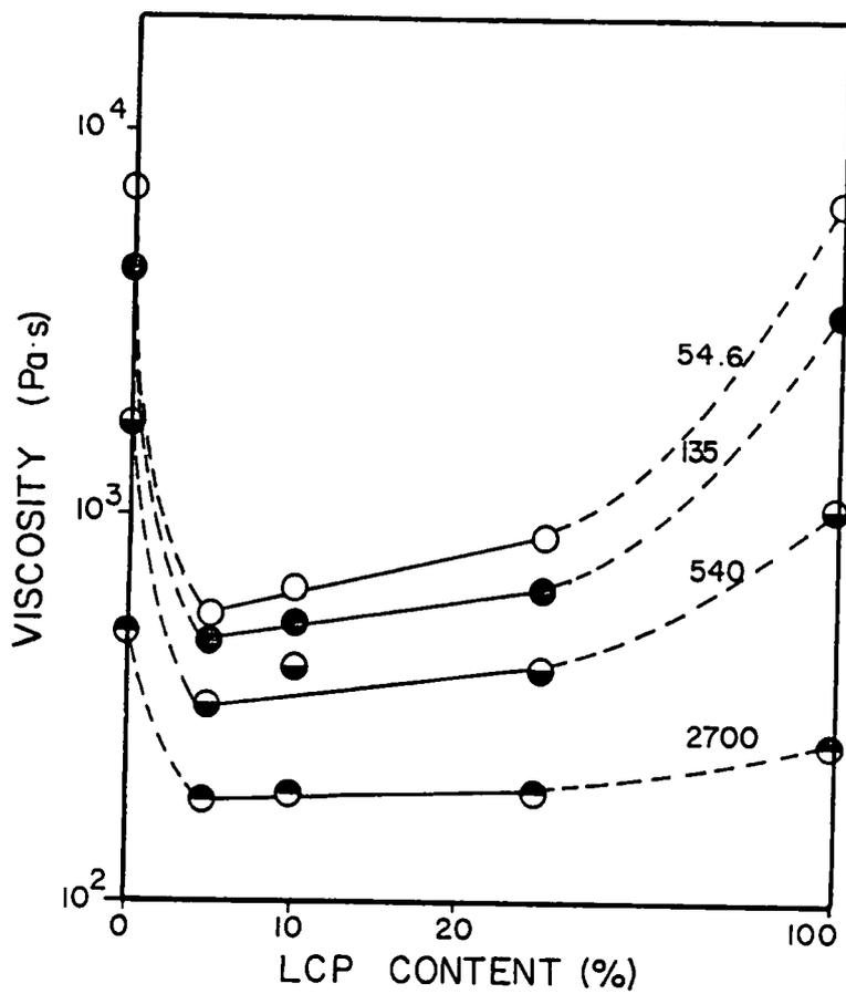
Figure 2.14. Composition dependence of LCP/PA blends as a function of shear rate at 260°C. From [80].
