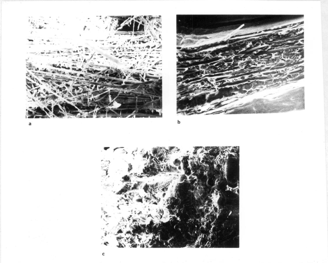
Figure 4.3. Micrographs of extruded 30% LCP blends after extraction of PC. a, 0.1588 cm x 8.89 cm die used; b, 0.3175 cm x 15.24 cm die used; c, no die or breaker plate used. 480 x.
