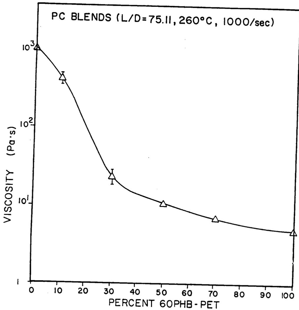
Figure 4.21. Viscosity of PC blends at 1000/sec as a function of composition from the ICR.
