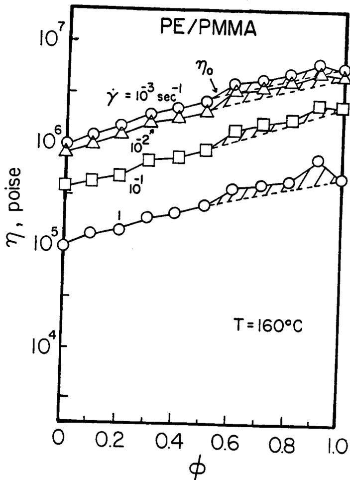
Figure 2.10. Dependence of viscosity on composition for several shear rates for PE/PMMA blends. From [48].
