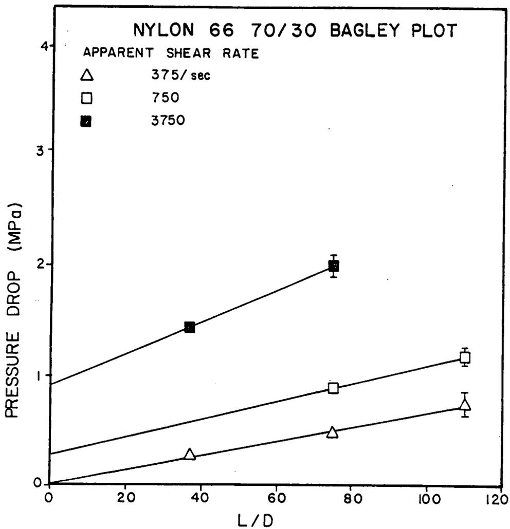
Figure B.8. Bagley Plot for 70/30 N66/LCP at 275°C.
