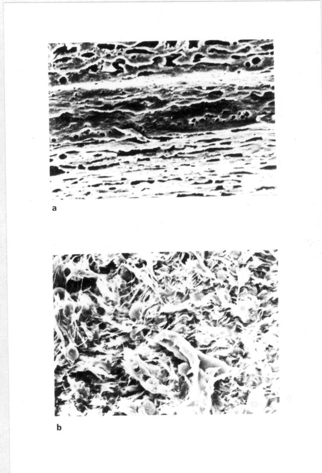
Figure 4.5. Micrographs of extruded 50% LCP after extraction of N66. 480 x.
