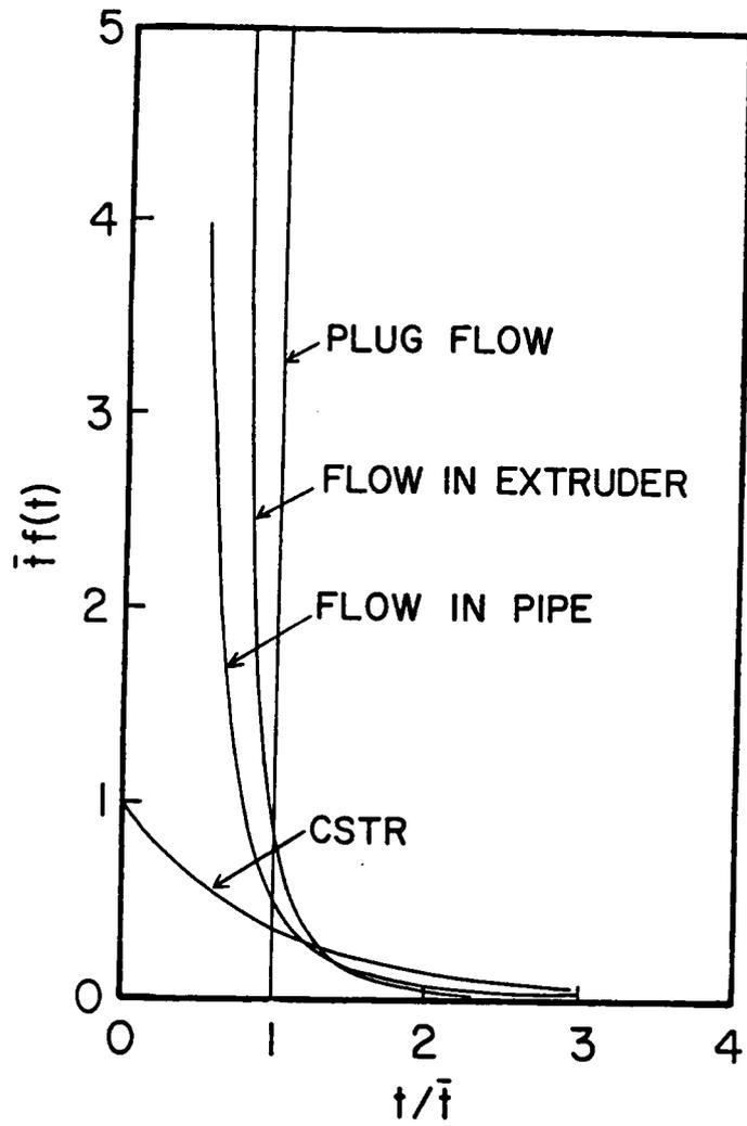
Figure 2.19. The residence time distribution function versus reduced time for various flows for isothermal flow of a Newtonian fluid. From [77].
