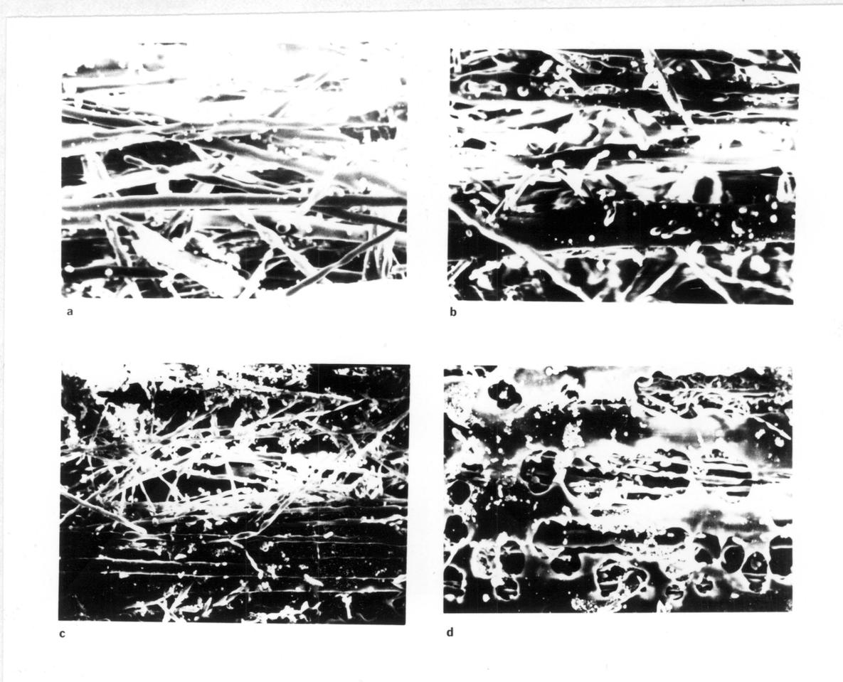
Figure 4.10. Micrographs of 30% LCP after extraction of PC. Samples extruded through ICR with capillary diameter of 0.178 cm and L/D of 7.82. a, 45.7/sec; b, 137/sec; c, 457/sec, center of sample; d, 457/sec, edge of sample. 480 x.
