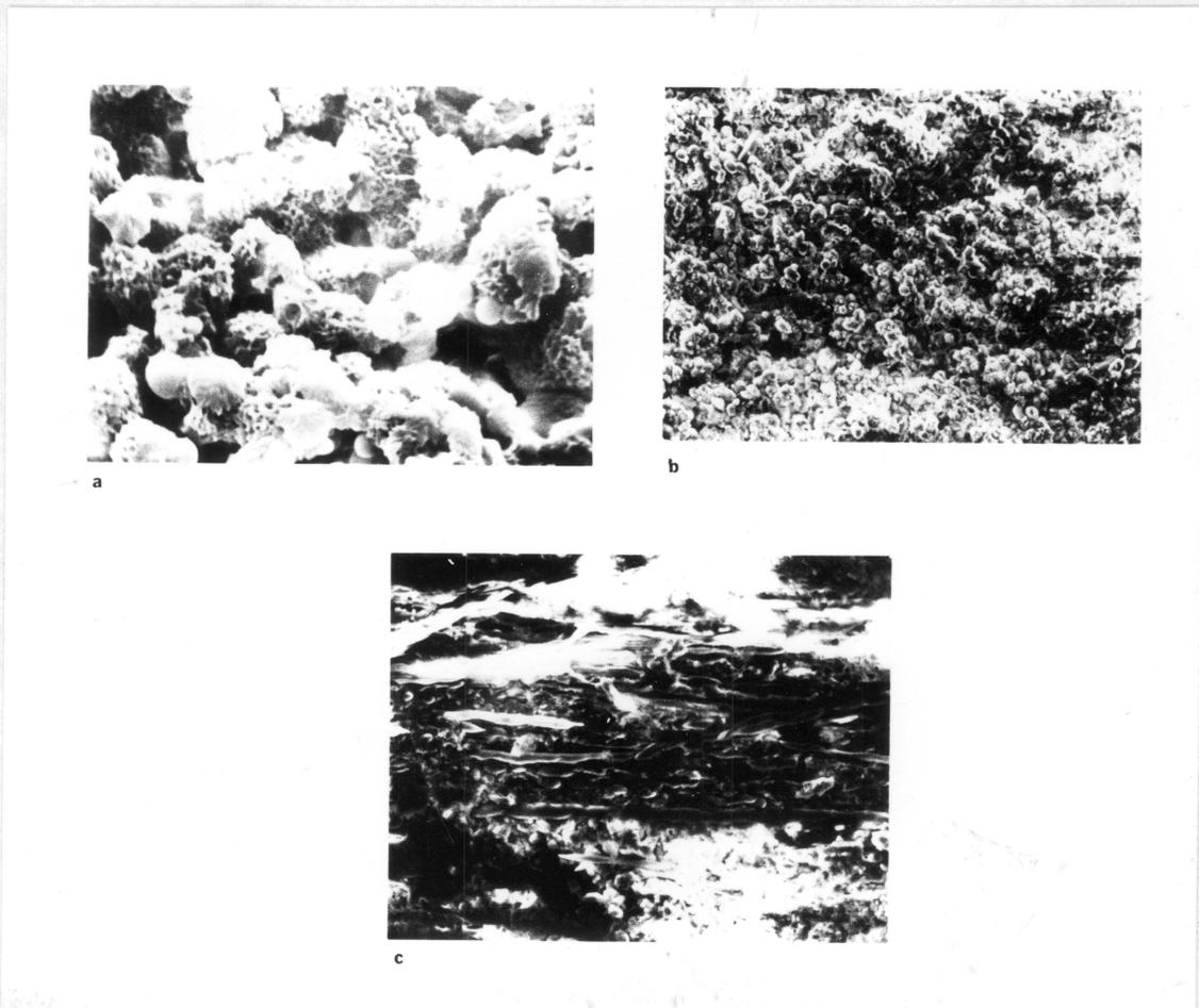
Figure 4.12. Micrographs of 30% LCP extruded through ICR with L/D of 40 after extraction of PC. a, 45.7/sec at 4800 x; b, 137/sec; c, 457/sec. b and c at 480 x.
