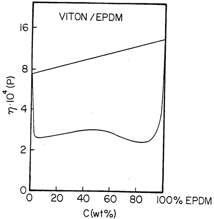
Figure 2.5. Viscosity as a function of concentration for a VITON/EPDM blend. From [45].
