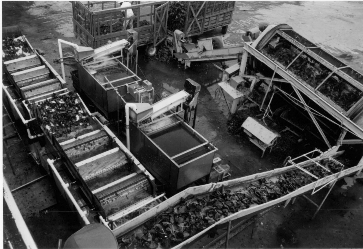
Figure 4: Overhead view of washing system adjacent to Exmore Plant. Rotary sand tumbler and conveyor into plant are at right and foreground (After Robinson,1976).
