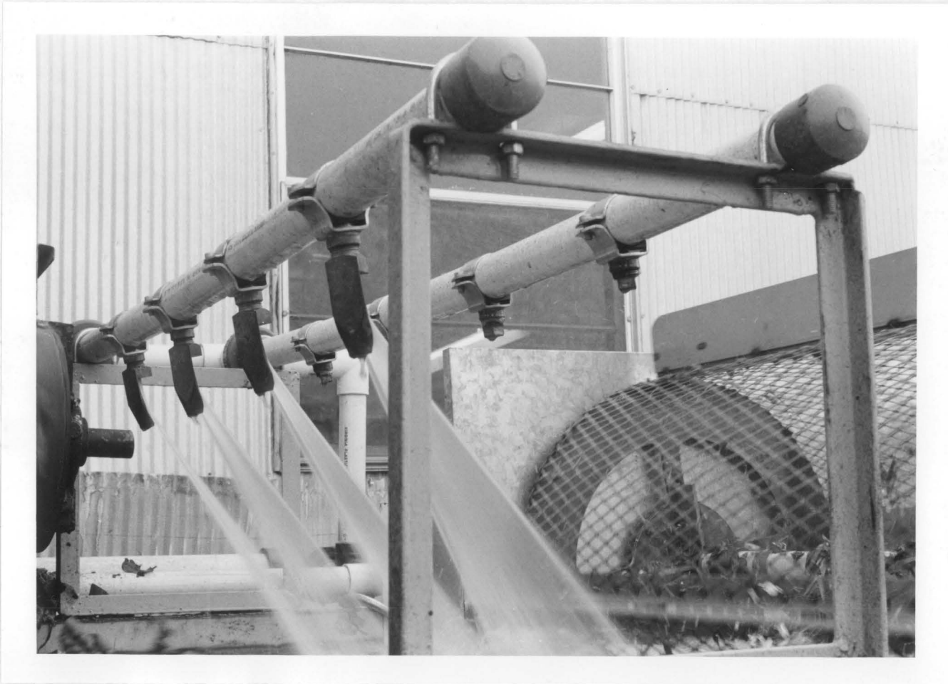
Figure 11: Water streams from the nozzles of the prototype washer.
