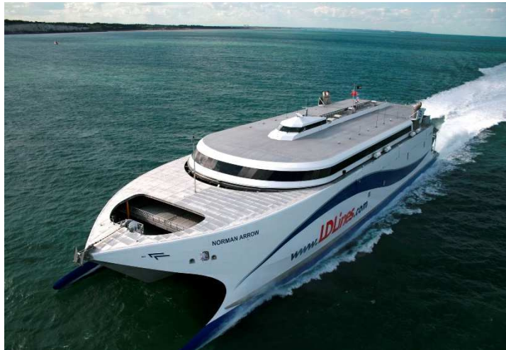
Figure 1. Modern high speed vessel constructed using aluminum hull and superstructure [73].
