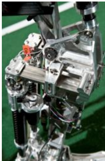
Figure 3-4. Titanium compliant members in series with the two ankle actuators.
