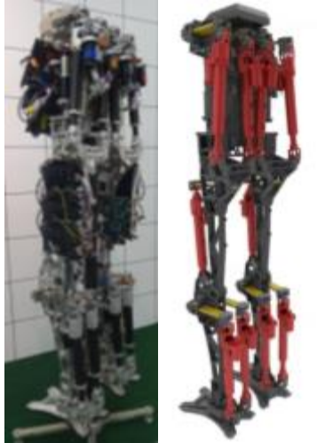
Figure 3-3. Linear actuators shown in red against SAFFiR's structure. Compliant beams shown in yellow.
