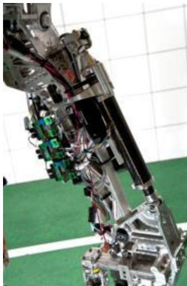
Figure 3-7. Details of knee actuator.
