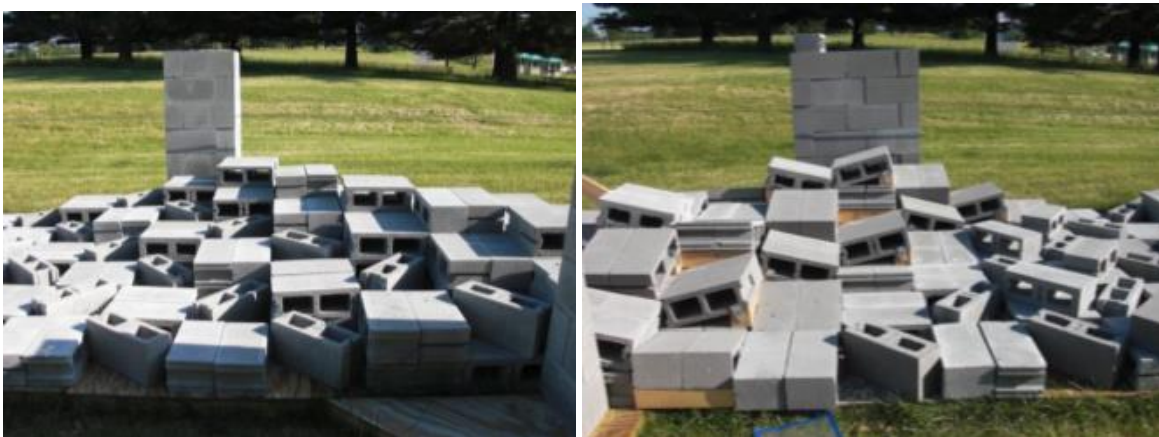
Figure D-3. Declined flat blocks on left and inclined Pitch/Roll blocks on right.
