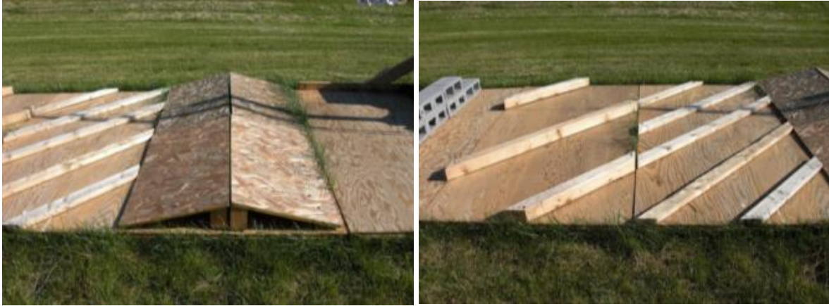
Figure D-1. The second and third portions of the DRC walking course. On left is the inclined ramps (2), and on right are the tripping hazards (3).
