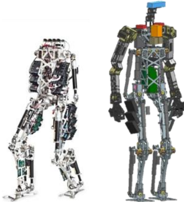
Figure 3-1. Currently state of completion of SAFFiR on left and proposed final CAD model.
