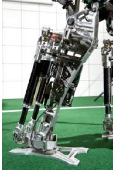
Figure 3-8. Parallel ankle actuation.
