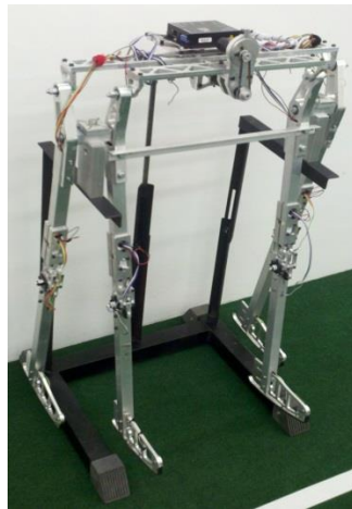
Figure 1-3. Passive Dynamic bipeds emphasize the natural dynamics of walking, in some cases by employing force control actuators.
