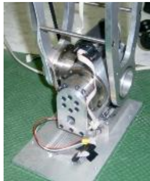
Figure 2-2. 2-DOF ankle joint of HUBO.
