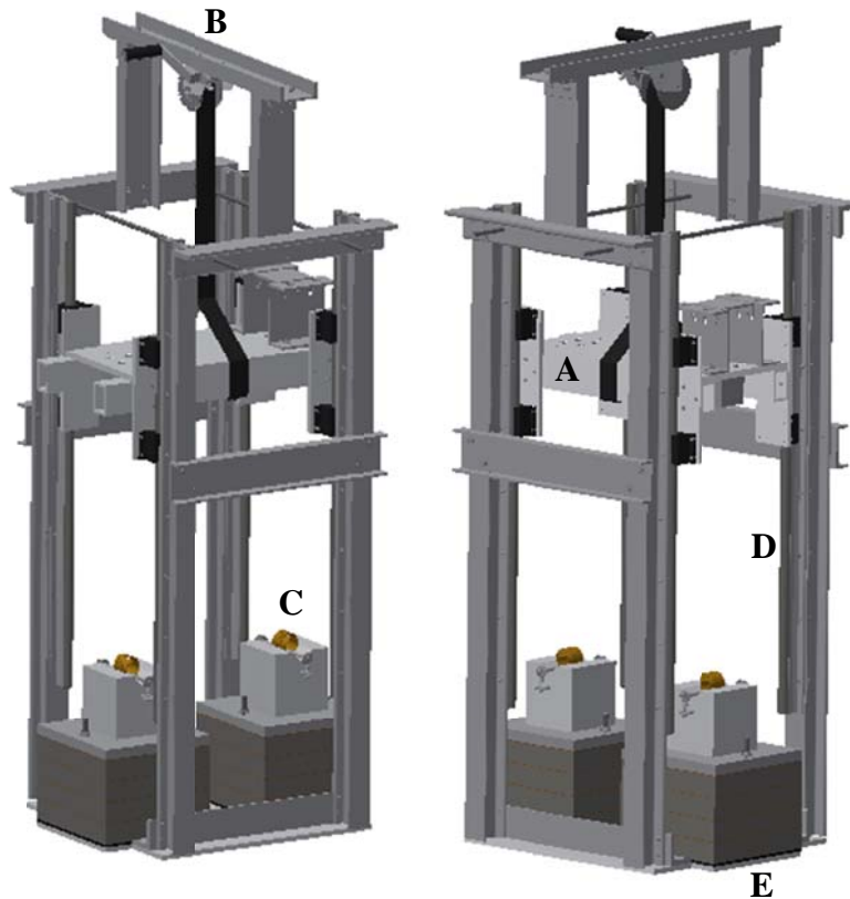
Figure 2.1: Translation-input injury device.
